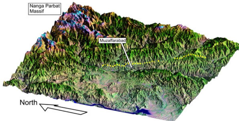
Figure 2.7: 3D perspective view of the Kashmir earthquake region and Muzaffarabad. The image is formed by draping LANDSAT 7 imagery over NASA SRTM (Shuttle Radar Topography Mission) digital topography. The fault identified by radar imagery is marked as a yellow dotted line. The mountains are higher on the far (north-eastern) side of the fault. (Source: COMET, 2005)
