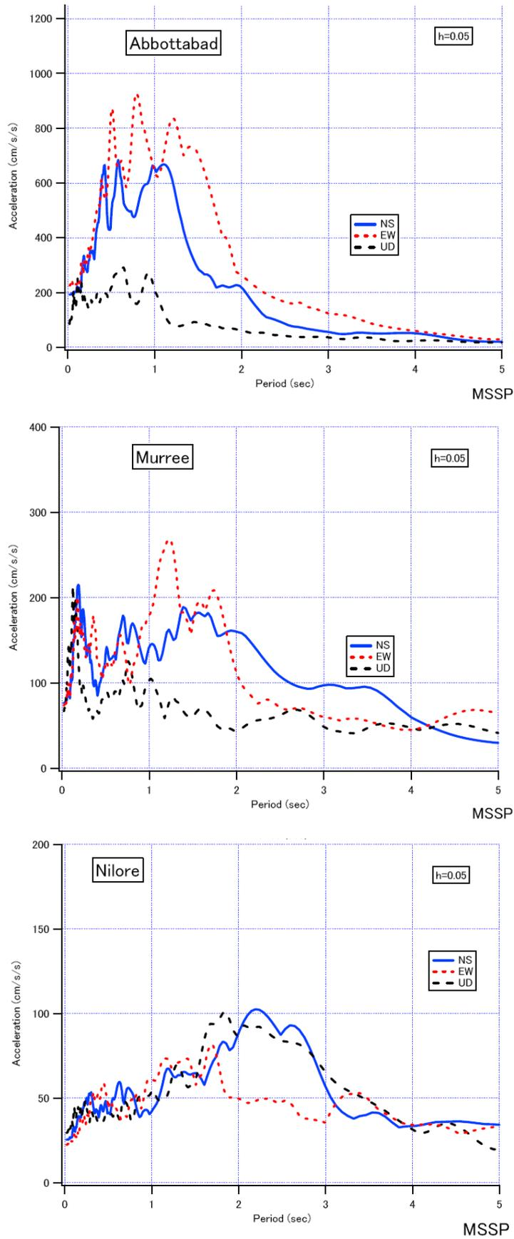
**Figure 2.11: Response spectra of ground motions (5% damped, elastic) recorded at Abbottabad, Murree and Nilore (Chaudury, 2006)**
