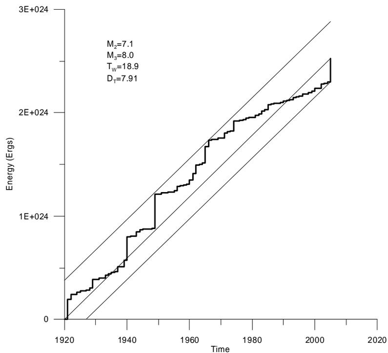
**Figure 2.16: Cumulative Strain Energy Release (CSER) for non-probabilistic modelling of seismicity and estimation of maximum credible earthquake in a region. The region occupies  $10^\circ$  of latitude and longitude centred on the Kashmir 2005 earthquake epicentre: a) excludes the Kashmir earthquake and b) includes the Kashmir earthquake as the last step in the energy release staircase (after Burton and Cole, 2006)**
