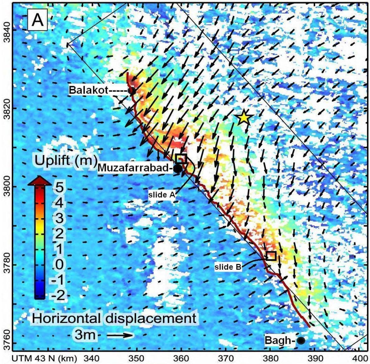
Figure 4.2: Displacement of the Earth's crust caused by the Kashmir 2005 earthquake. Black arrows indicate horizontal displacement and colour vertical uplift, the star indicates the epicentre (adapted from Pathier *et al.*, 2006). Significant landslides discussed in the text occurred at "slide A" (Muzaffarabad slide) and at "slide B" (Hattian slide)
