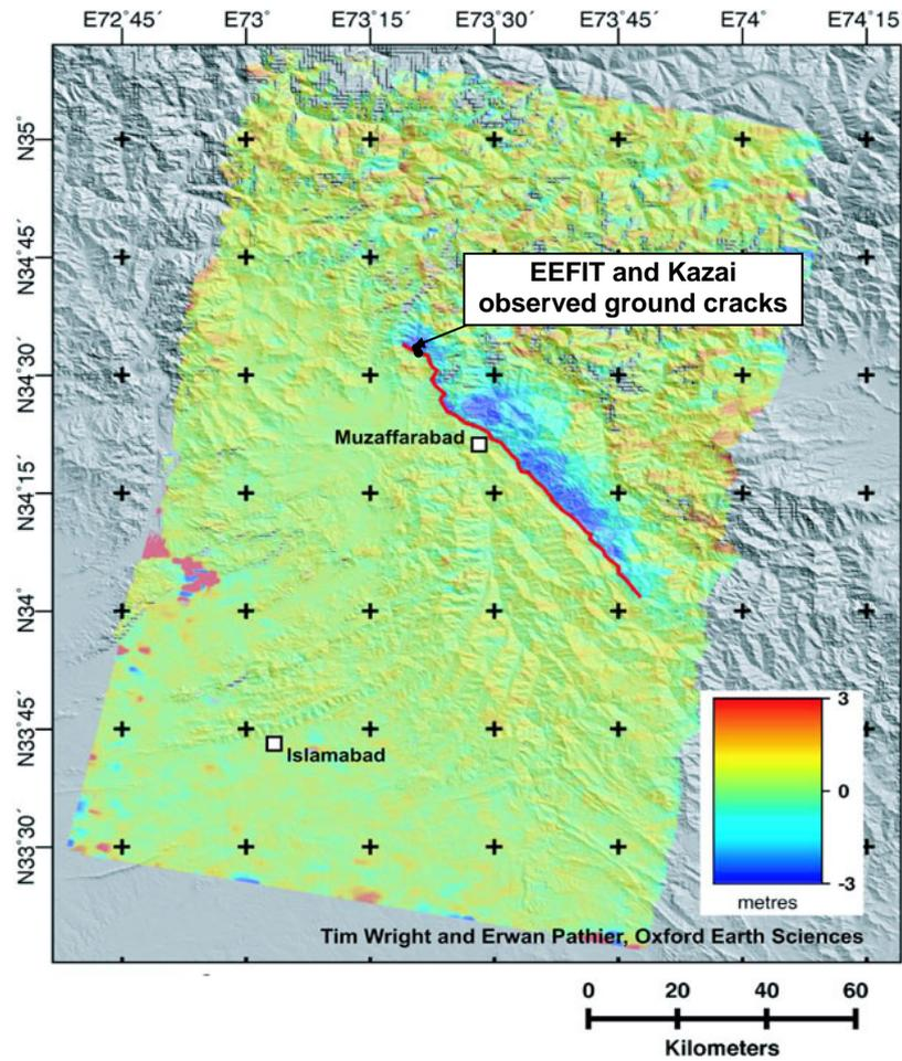
Figure 2.6: Map showing the location of the causative fault of the October 8, 2005 earthquake (Source: COMET, 2005)
