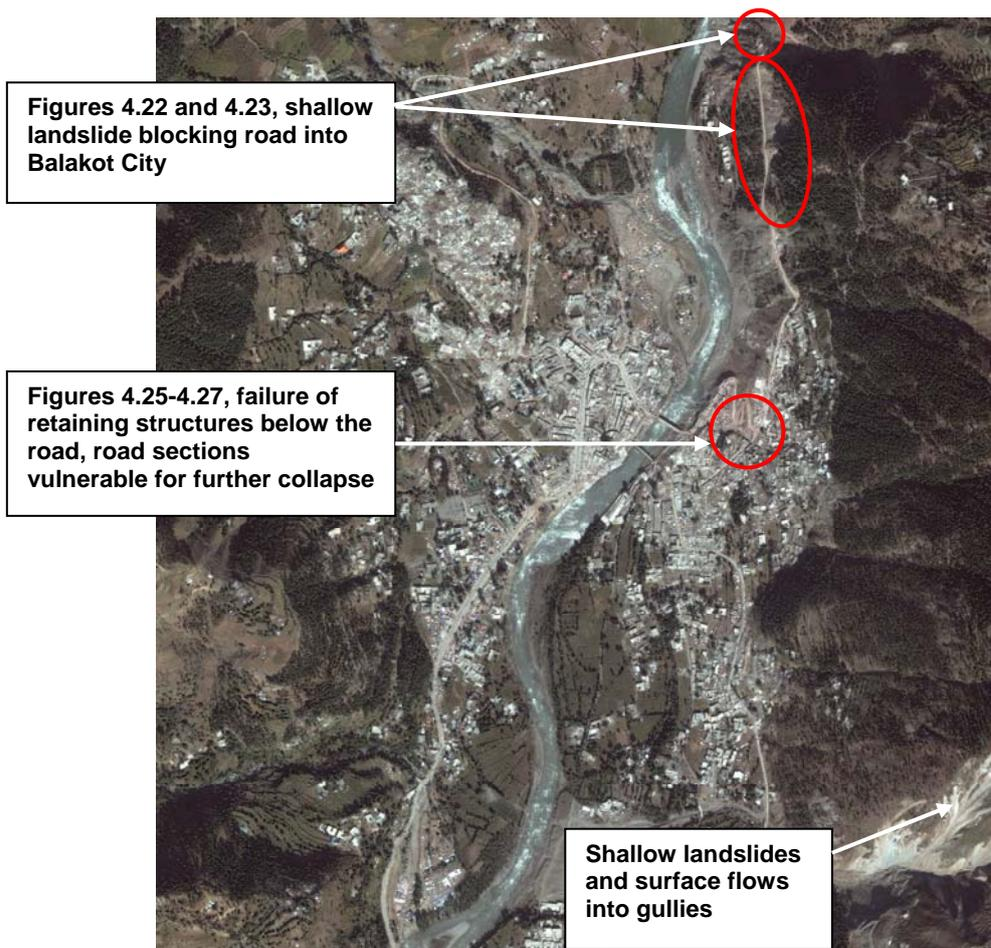
Figure 4.14: Location of landslides and ground failures in Balakot City (Digital Globe, 2005)
