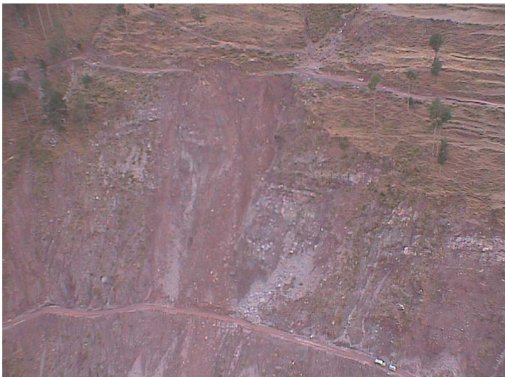
**Figure 4.43: Agricultural terraces slipping down steep terrain and valley-side road, all threatened by landslide, near Dhanni Nelam (Dhanni Nelam-Islamabad flight)**
