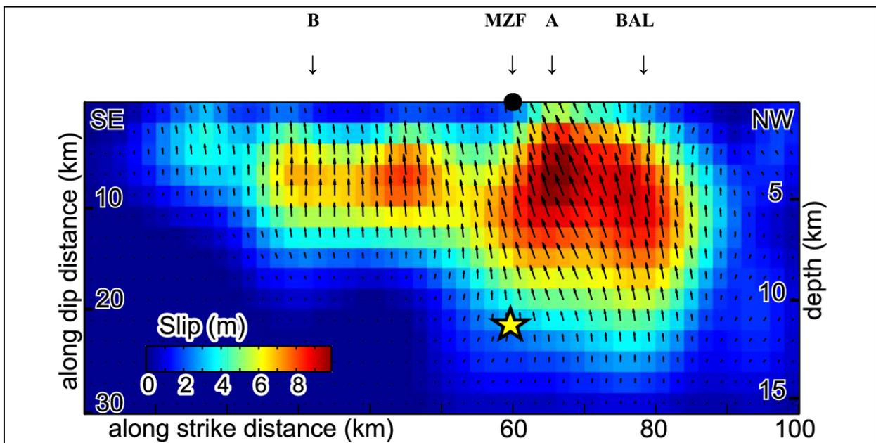
Figure 4.7: Slip distribution mapped in the fault plane (after Pathier *et al.*, 2006): BAL = Balakot; MZF = Muzafarrabad. Position A = Chela Bandi, Muzafarrabad slide seen in Figures 4.4, 4.5 and 4.6 and position B = Hattian slide as seen in Figures 4.8, 4.9 and 4.10
