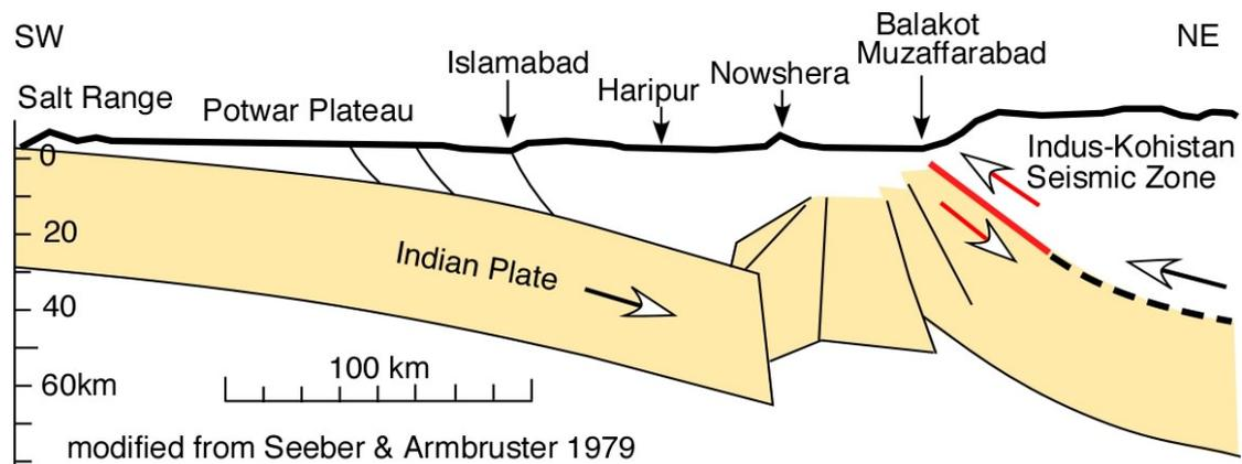
Figure 2.5: Cross-sectional view of the rupture area in the Indus-Kohistan Seismic Zone
