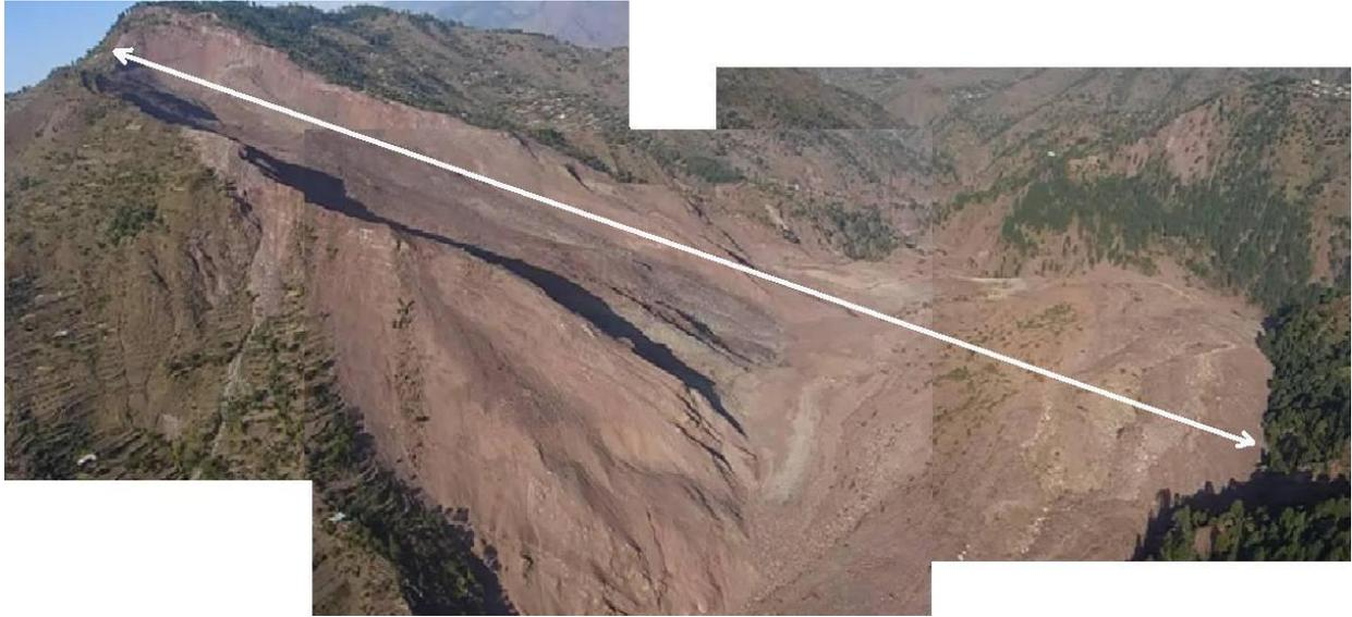
**Figure 4.9: The Hattian slide, Pir Punjal Mountains: the major landslide in the Kashmir 2005 earthquake. This deep cutting landslide from source scarp to toe (white arrow) stretches over approximately 2,850 m (photo collage by Charles Scawthorn)**
