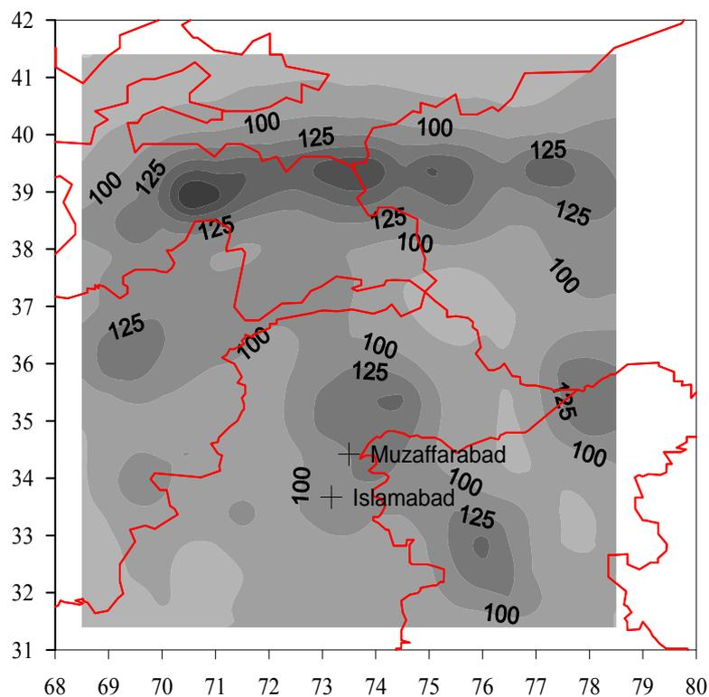
**Figure 2.14: Ground shaking seismic hazard map for Kashmir using Sharma's (1998) attenuation law. The contours are expected maximum peak ground accelerations in  $\text{cm s}^{-2}$  with a one-in-ten chance of being exceeded during 50-years (extracted from Burton and Cole, 2006)**
