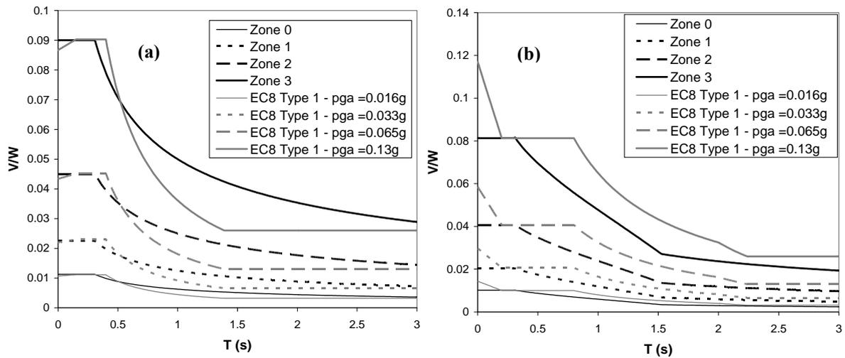
**Figure 6.3: Examples of the plots of normalized base shear vs building fundamental period given by the Pakistan 1986 Seismic Code and Eurocode (EC) 8 used to find the PGA corresponding to each seismic zone: (a) Normal importance, non-ductile frame and rock-site conditions, (b) Normal importance, ductile frame and soil conditions**
