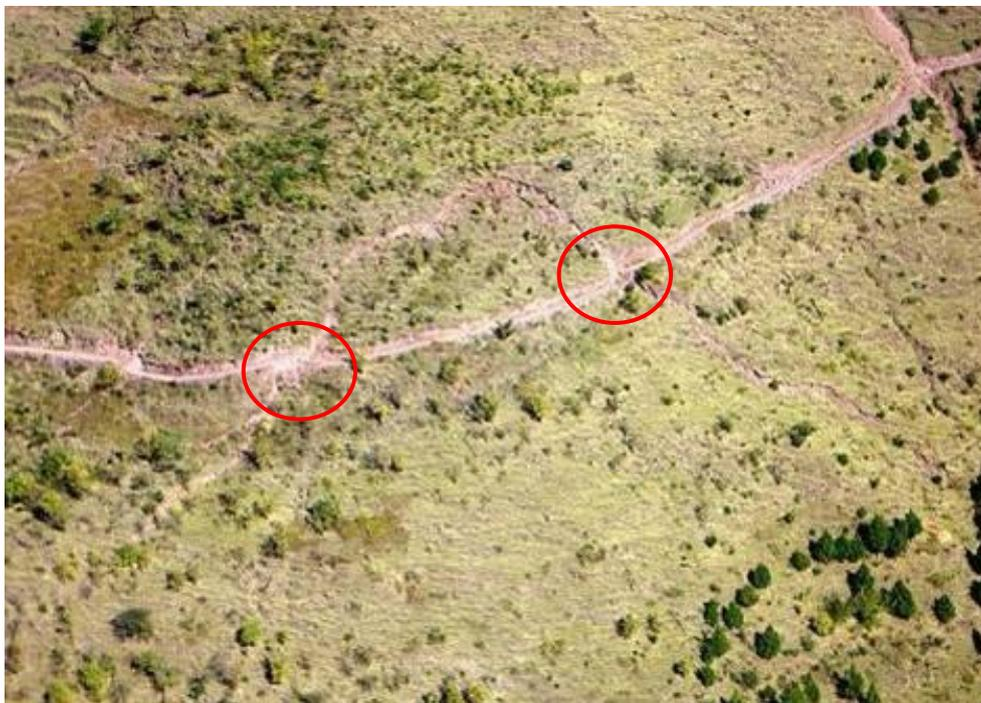
**Figure 4.36: Incipient landslide threat to road: the road is cut in two places by cracking (photo by Charles Scawthorn)**
