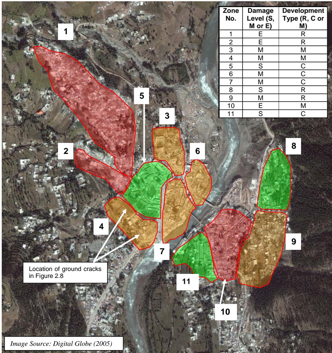
Figure 3.10: Selected damaged areas in Balakot city
