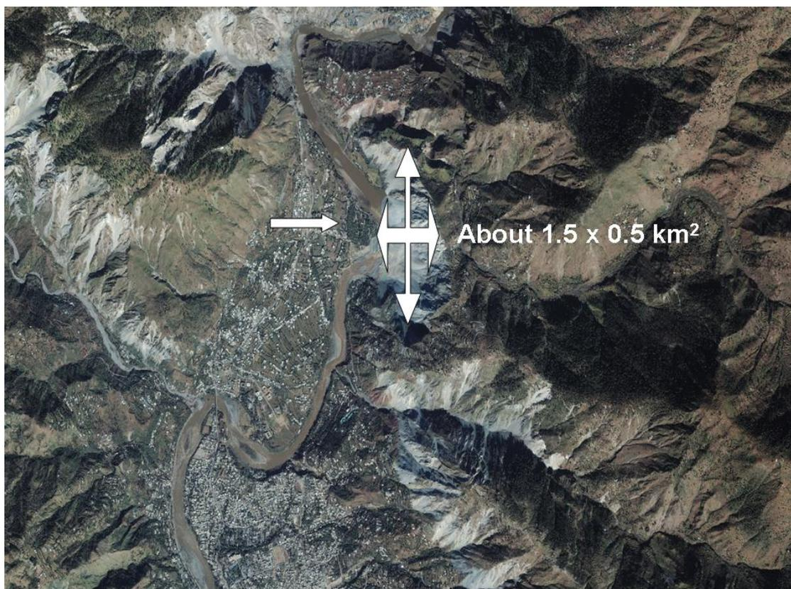
Figure 4.6: Main landslide at Chela Bandi, north of Muzafarrabad, imaged from space (Image NASA) with extent 1.5 km N-S and 0.5 km E-W. Arrow to the left indicates point of view in photographs of Figures 4.4 and 4.5
