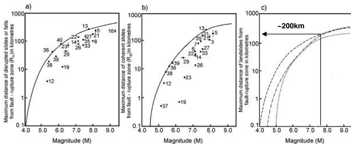
**Figure 4.1: Relationships between maximum distance of landslides from causative fault and earthquake surface wave magnitude: a) disrupted slides and falls, b) coherent slides, c) envelopes to a) and b) and lateral spreads (dotted line) (after Keefer, 1984)**
