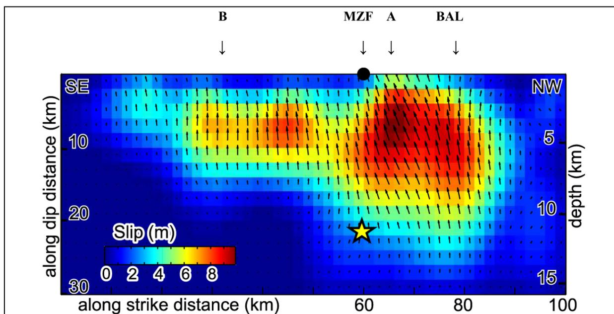
Figure 4.7: Slip distribution mapped in the fault plane (after Pathier *et al.*, 2006): BAL = Balakot; MZF = Muzafarrabad. Position A = Chela Bandi, Muzafarrabad slide seen in Figures 4.4, 4.5 and 4.6 and position B = Hattian slide as seen in Figures 4.8, 4.9 and 4.10
