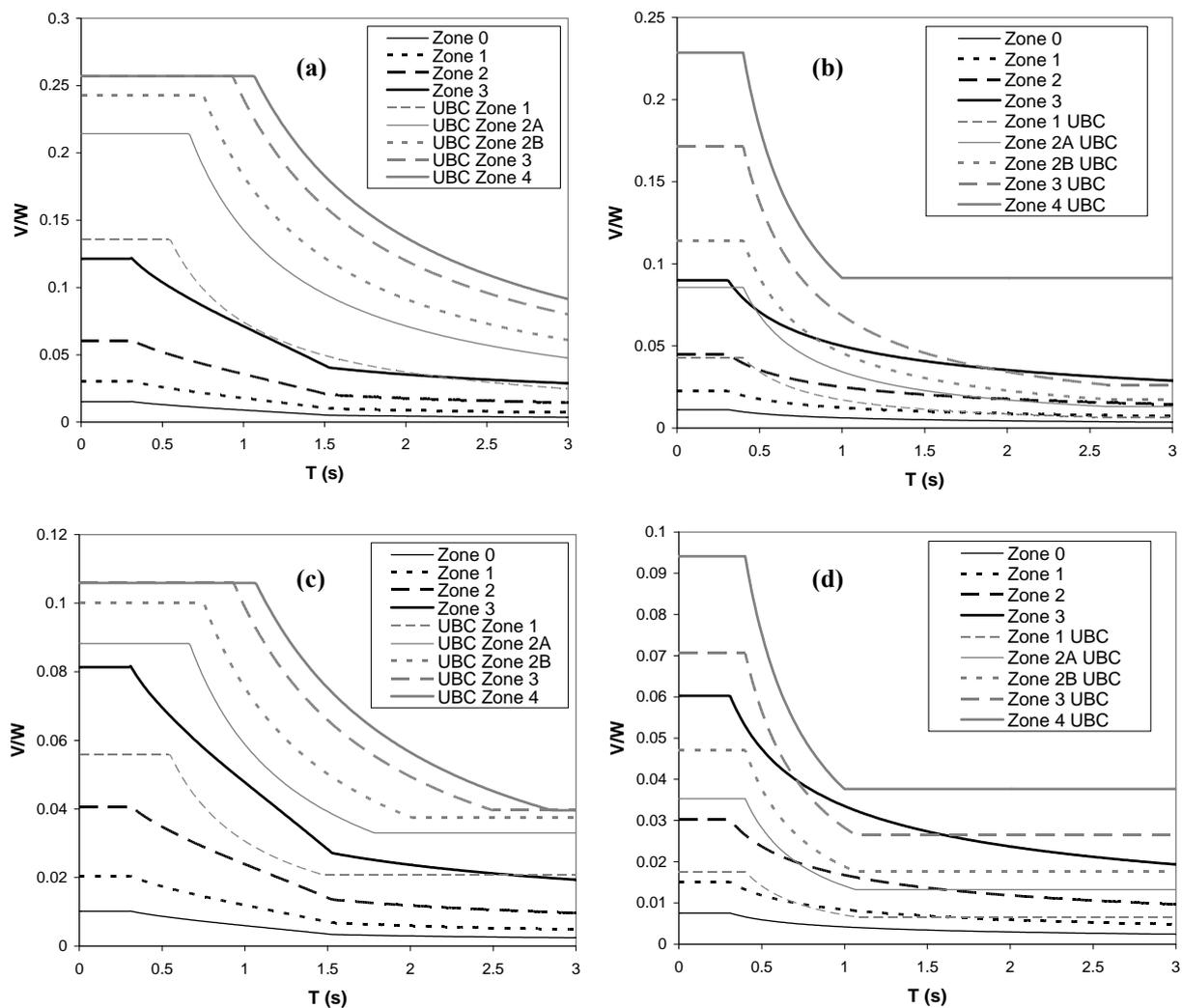
**Figure 6.4: Examples of the plots of normalized base shear vs building fundamental period given by the Pakistan 1986 Seismic code and UBC 1997: (a) Normal importance, non-ductile MRF and soft-soil site conditions, (b) Normal importance, non-ductile MRF and rock site conditions, (c) Normal importance, ductile MRF and soft-soil site conditions, (d) Normal importance, ductile MRF and rock site conditions**
