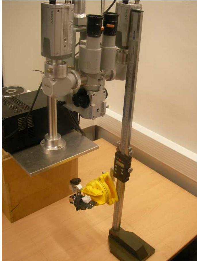
Figure 4.17: Stereoscopic surgical microscope and rotational gauge experimental setup.
