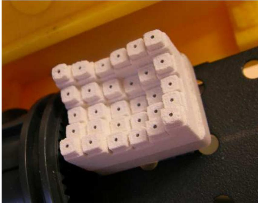
Figure 4.9: 3D non-coplanar calibration object manufactured with 3D Zprinter<sup>®</sup> 450 - Z Corporation.
