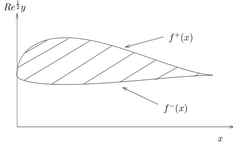
Figure 3.2: A typical aerofoil showing the definitions of  $f^+(x)$  and  $f^-(x)$ .
