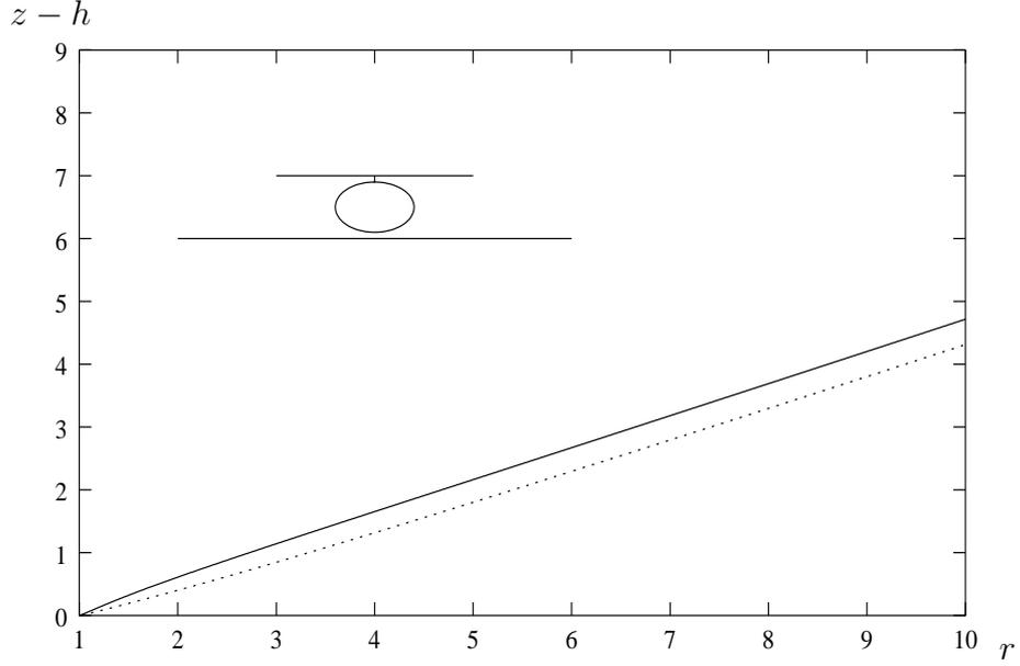
Figure 2.7: Comparison of the layer shapes for a disc at a height  $h = 1$  with and without a spherical body shape. The body shape is shown and has a radius of 0.4. The solid line is the layer shape with the body present.
