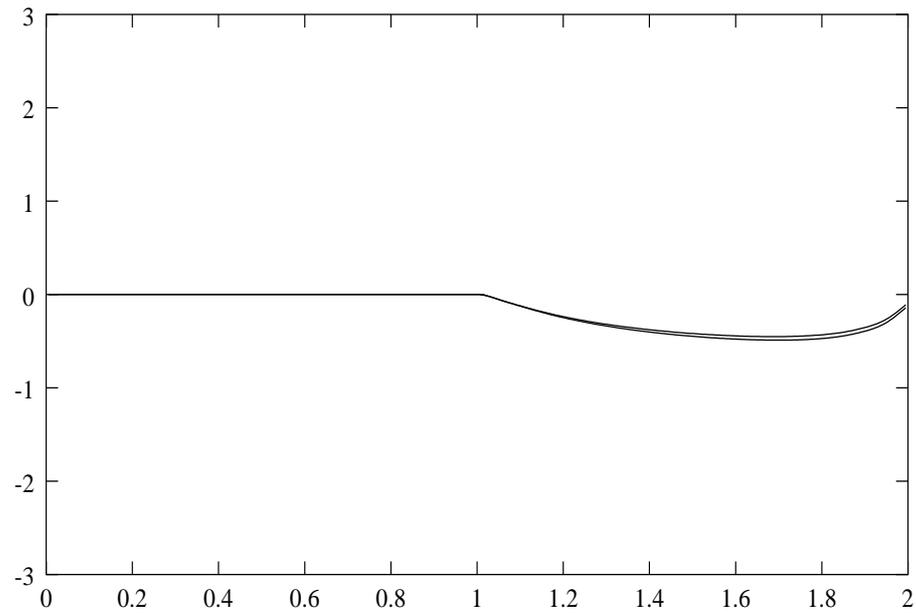
Figure 4.7: Comparison between the wake shapes  $s(x)$  for the current periodic method and blade 4 of the five blade case from chapter 3 for  $h = 0.0625$ . The shape from this chapter is the lower of the two.
