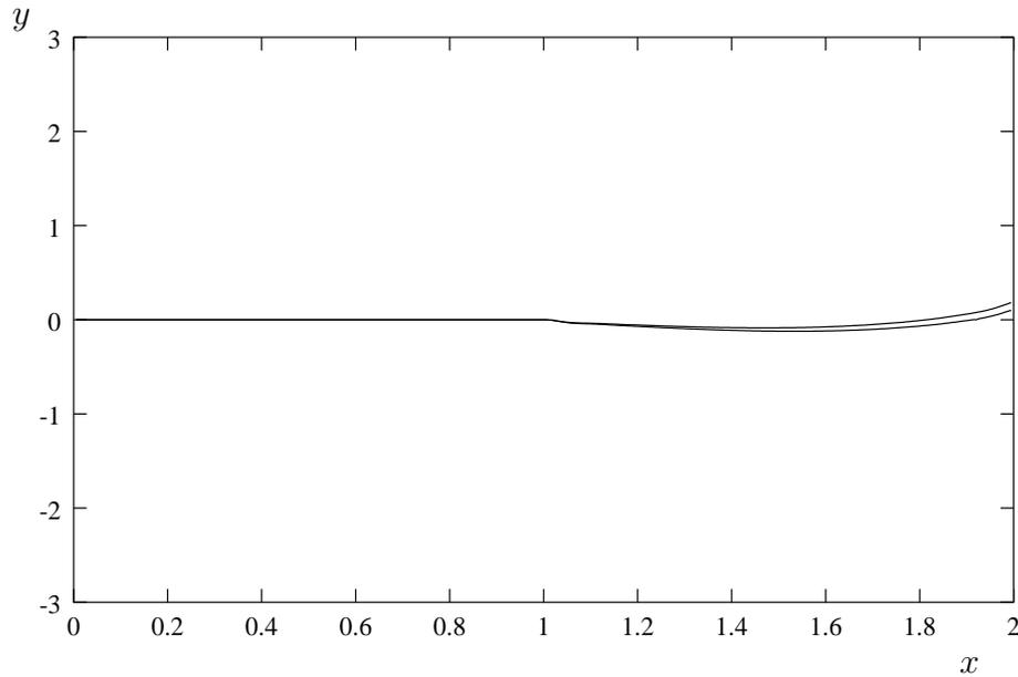
Figure 4.6: Comparison between the wake shapes  $s(x)$  for the current periodic method and blade 4 of the five blade case from chapter 3 for  $h = 0.25$ . The shape from this chapter is the lower of the two.
