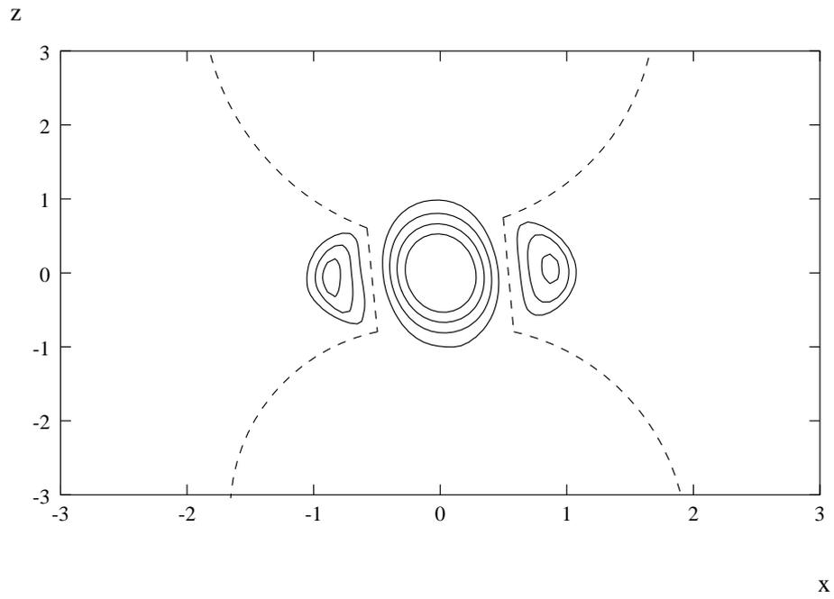
Figure 6.4: Contour Plot of the Pressure solution. The dashed line corresponds to  $P = 0$ . Between the lines  $P < 0$  and  $P$  is positive elsewhere. The contour intervals are 0.02
