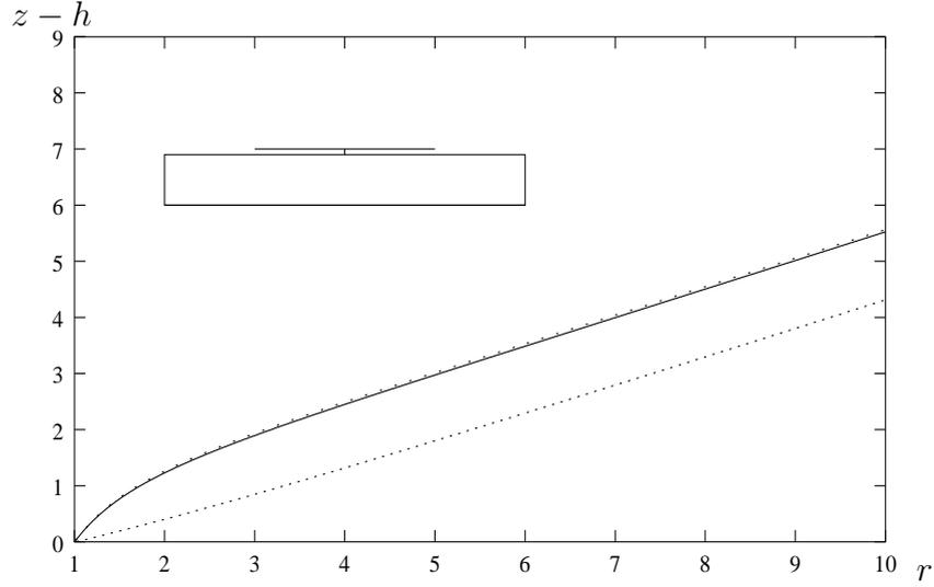
Figure 2.8: Comparison of the layer shapes for a disc at a height  $h = 1$  with and without a large cylindrical body shape. The solid line is the layer shape with the body present while the lowest line is the disc without any body shape and the top line is a disc with no body shape but at a height  $h = 0.1$  (the length of the stem joining the disc and cylinder)
