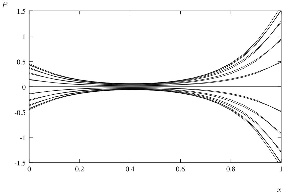
Figure 5.2: A sample pressure solution, varying in  $x$  for various  $z$  values, with  $L_1 = 1$ ,  $L = 1$  with  $J = \sin(\frac{2\pi z}{L_1})$ ,  $K = \cos(\frac{2\pi z}{L_1})$ ,  $\delta = \sin(\frac{2\pi z}{L_1})$
