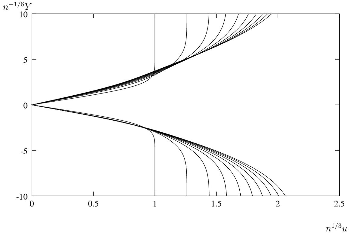
Figure 4.2: The scaled  $u$  velocity profiles mid-blade in the boundary layer for a ten blade case. Note the near periodicity for small  $y$  and the gradual growth for large  $y$ . The scales used are those determined below for the innermost layer.
