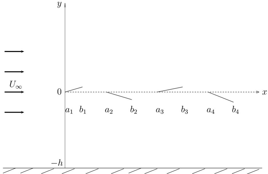
Figure 3.1: The flow configuration of  $n(= 4$  here) blades at a distance  $h$  above horizontal ground.
