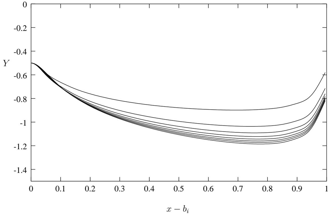
Figure 4.4: A Comparison of the wake-center line shapes for a ten blade case. The uppermost line is wake one, the lowermost wake nine. Notice the near periodicity as increasingly more blades are passed.
