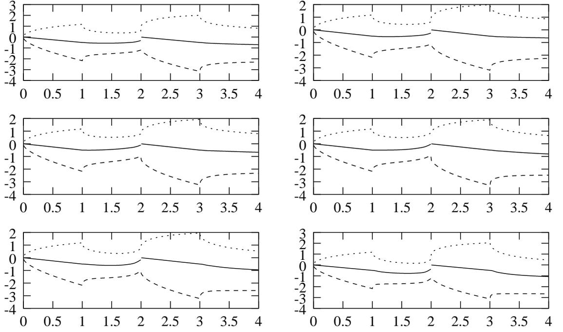
Figure 3.14: Displacement thicknesses  $\delta^\pm(x)$  and wake shapes  $s(x)$  for two blades at negative angle of attack for heights  $h = 2$  to  $h = 0.0625$  as in figure 3.11.
