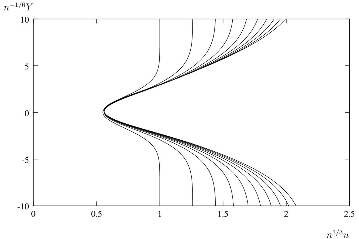
Figure 4.3: The scaled  $u$  velocity profiles mid-wake in the boundary layer for a ten blade case. Note the near periodicity for small  $y$  and the gradual growth for large  $y$ . The scales used are those determined below for the innermost layer.
