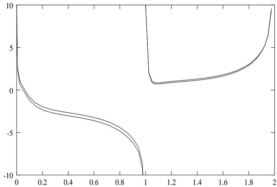
Figure 4.8: Comparison between the underneath pressures  $p^-$  for the current periodic method and for blade 4 of the five blade case from chapter 3 for  $h = 0.25$ . The shape from this chapter is the lower of the two.
