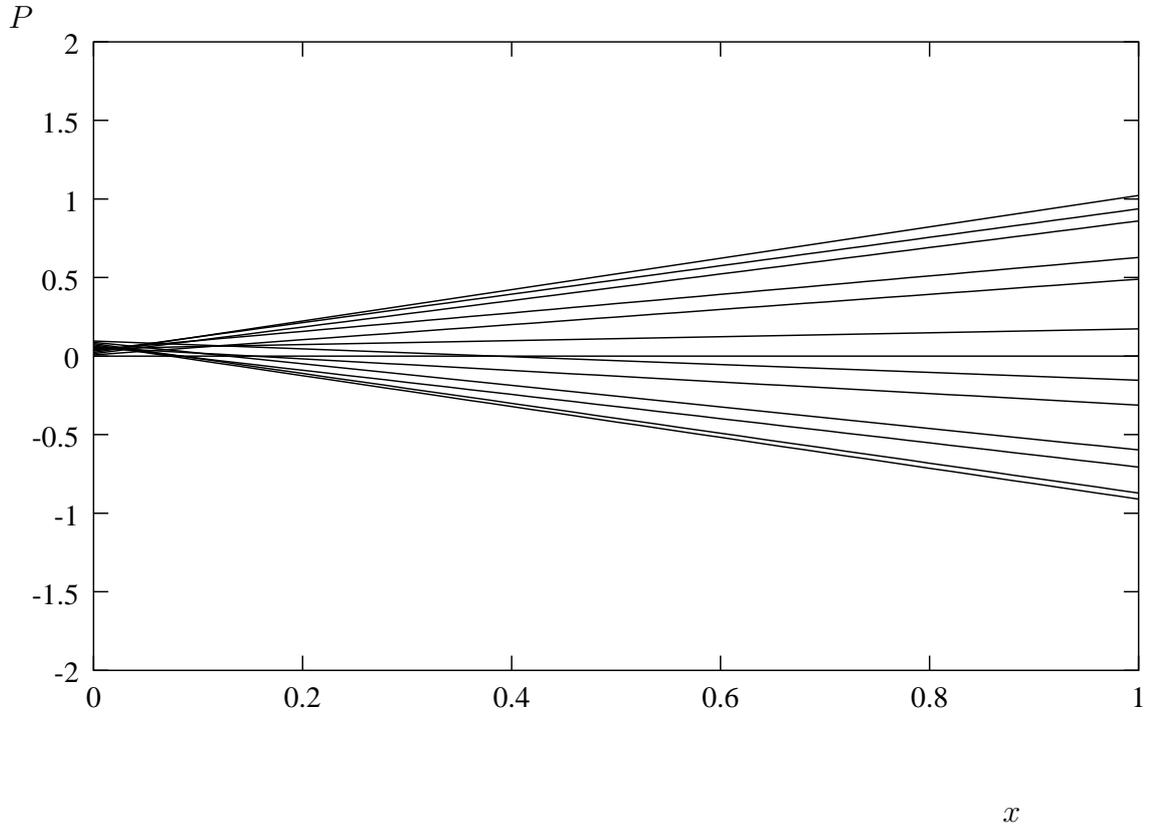
Figure 5.3: A sample pressure solution, varying in  $x$  for various  $z$  values, with  $L_1 = 20$ ,  $L = 1$  with  $J$ ,  $K$ ,  $\delta$  as in figure 5.2. Note the pressure solution is nearly linear as suggested in the analysis in the text.
