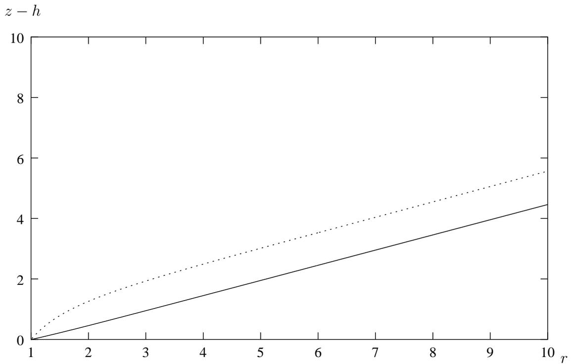
Figure 2.13: Comparison between the layer shapes for the pressure jump case (solid line) and the no pressure jump case (dotted line) for  $h = 0.1$  with  $\alpha = 1$ . Note the similarity in the linear layer shape for the pressure jump case here and for  $h = 0.3$  case in figure 2.12.
