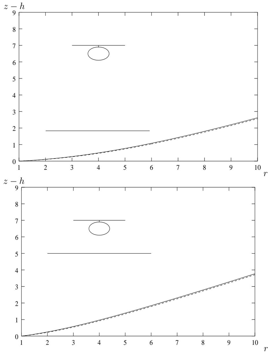
Figure 2.6: Comparison of the layer shapes for a disc with and without a spherical body shape at two different heights,  $h = 5$  and  $h = 2$ . The body shape is shown and has a radius of 0.4. The solid line is the layer shape with the body present.
