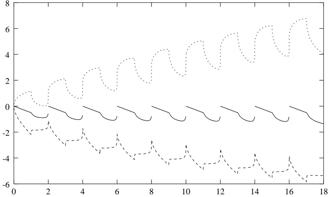
Figure 3.16: The wake centre line shapes and viscous displacements for nine blades at angle of attack. Note the near periodicity in  $s(x)$ .
