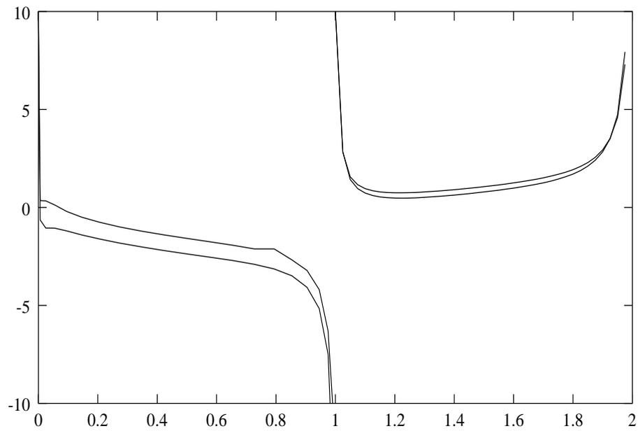
Figure 4.9: Comparison between the underneath pressures  $p^-$  for the current periodic method and for blade 4 of the five blade case from chapter 3 for  $h = 0.0625$ . The shape from this chapter is the lower of the two.
