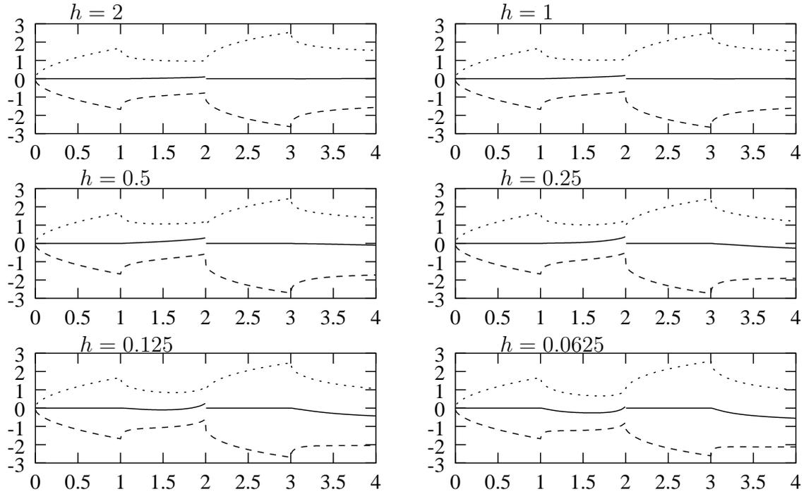
Figure 3.11: Displacement thicknesses  $\delta^\pm(x)$  and wake shapes  $s(x)$  for two flat blades.
