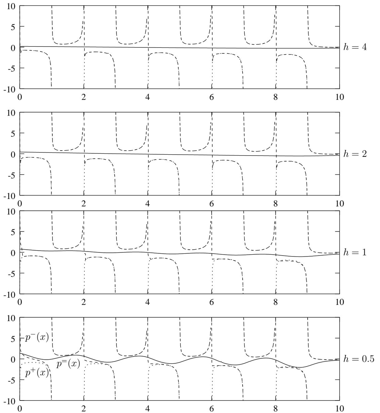
Figure 3.7: Plots of the above, below and ground pressures  $p^+(x)$ ,  $p^-(x)$  and  $p^{\bar{}}(x)$ , for the case of five flat blades, with  $h$  values ranging from  $h = 4$  to  $h = 1/2$ .
