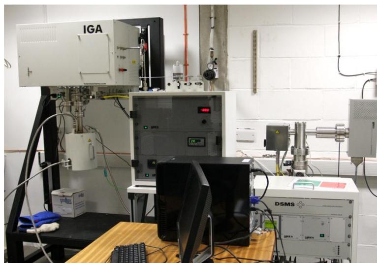
Figure 3-6 Intelligent Gravimetric Analyzer (IGA-003) combined with Mass Spectrometer.
