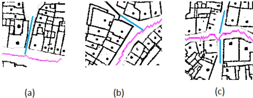
Figure 9.6: This figure shows three cases where the algorithm failed within the map. (a) and (b) Illustrates a junction where the entrance is too small. (c) Shows a “Cross” junction where neither roads leaving the current path is detected.
