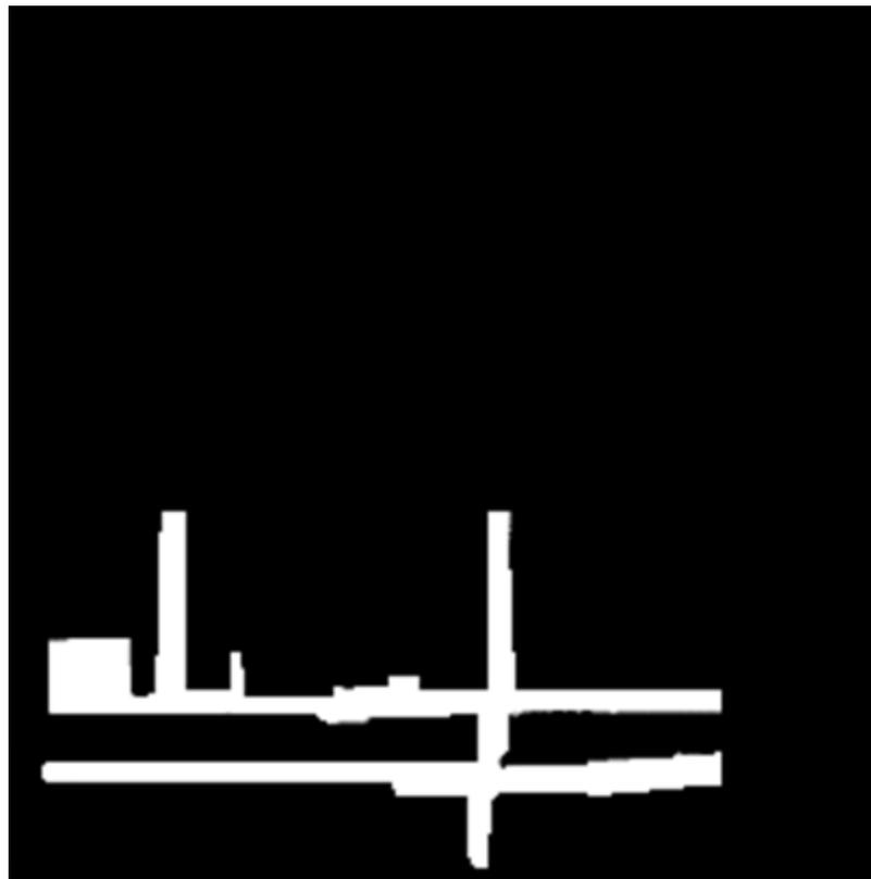
Figure A.14: This illustrates a typical input image for the Koblenz map. As the map contains many imperfections such as houses with the same colour as the road surface, To make the map suitable for the algorithm the houses were blacked out manually within Photoshop.
