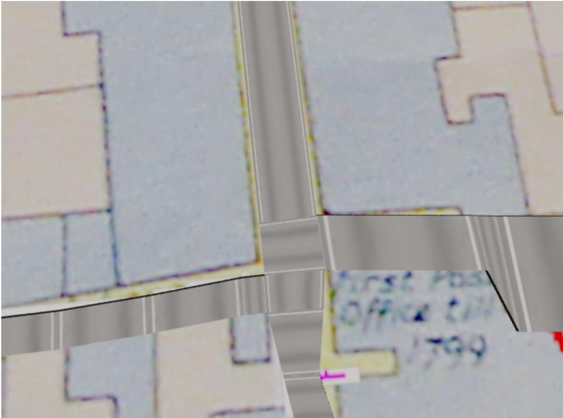
Figure 5.11: Screen dump showing how the texture errors appear when UVW mapping is applied per face, on a joined road network modelled by hand within 3ds max.
