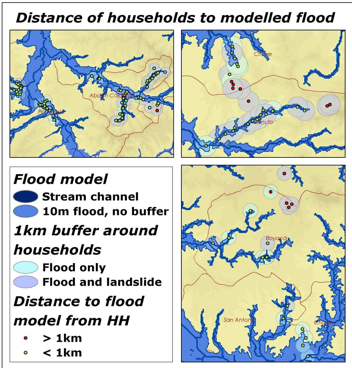
Figure 62. Households reporting occurrences of floods and distance to 10m flood model with no buffer
