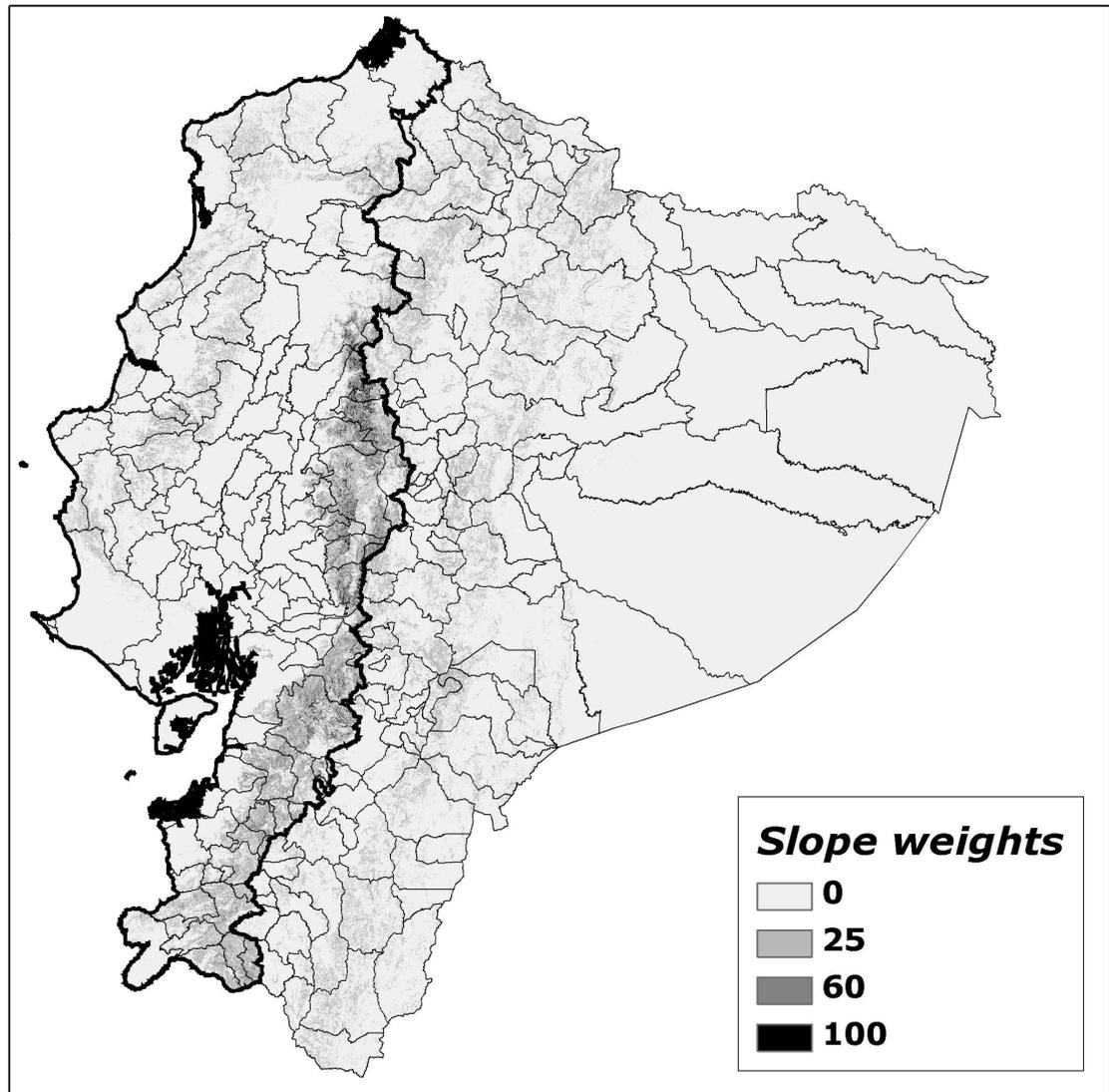
Figure 48. Landslide model using weighted slopes, soils and areas experiencing large rainfall amounts during El Niño events
