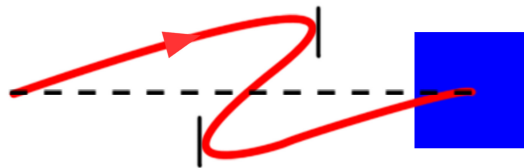
Figure 4.4: Orthogonal direction changes when navigating towards a target. The red line represents the path of the cursor and the blue square represents the target. The solid black lines identify where an ODC has occurred.
