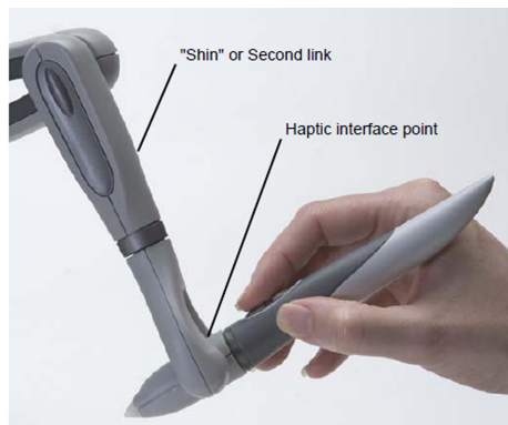
Figure 3: The HIP position on the Phantom Omni (adapted from Openhaptics Toolkit Programmer's Guide. [Teca])
