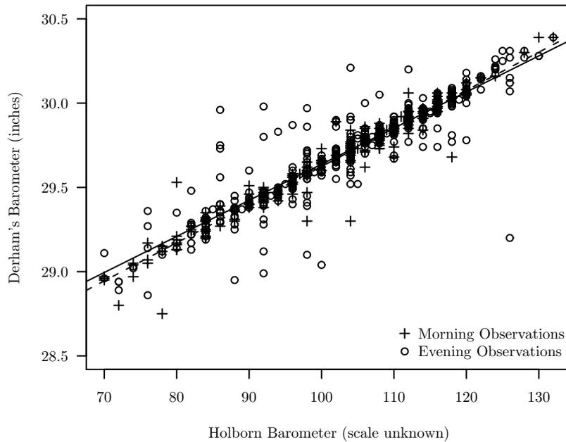
**Figure 2.6:** The relationship between the Holborn barometer and Derham’s barometer, 1704–6 (OS). Crosses indicate the morning readings and circles represent the evening readings. The dashed and filled lines show the least squares fit for the morning and evening readings respectively.
