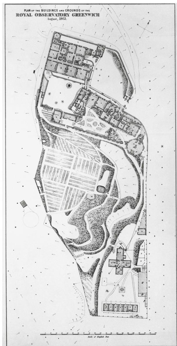
**Figure 2.9:** A map of the Royal Observatory, Greenwich in August 1863. The cross-shaped building (The Magnet House) in the bottom of the diagram housed the standard barometer until 1917. The building was constructed entirely of wood due to the magnetic observations also being observed there. In 1913–14 a new building was constructed adjacent to the Magnet House to which the standard barometer was transferred in 1917 (Dyson, 1932).
