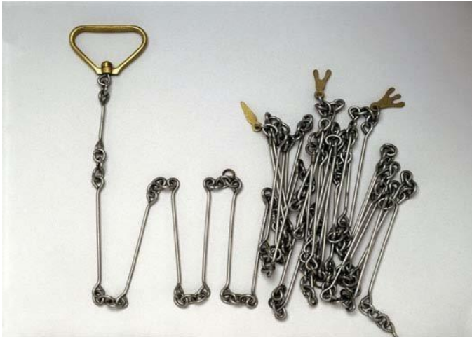
A typical image of a Gunter's land measuring chain.
