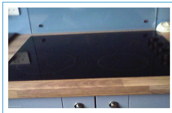
Figure 10. A glass, all black hob which made it difficult for a participant to use.
