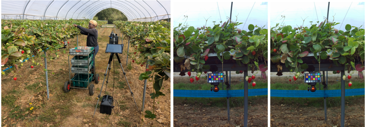
Figure 2: Acquisition experimental setup (left) and uncalibrated pipeline output of initial image (middle) then after ripe fruit harvested (right).
