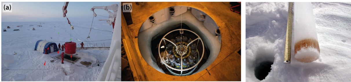
Figure 2.6: Left and middle: Images from the MOSAiC CTD sampling site, including a CTD rosette being lowered into the sea, adapted from [7]. Right: An example ice core, from [119]. The brown ‘stripe’ is from the sea-ice interface, and comprised of a dense algal layer.
