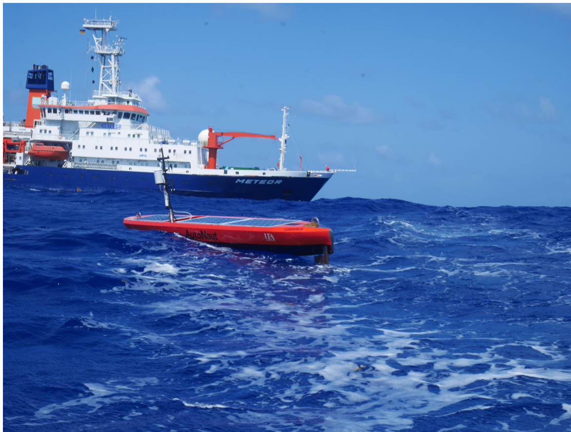
Figure 2.1: Photograph of Caravela (an AutoNaut vessel) in front of the German R/V Meteor during the EUREC 4 A campaign. (Credit: Callum Rollo.)
