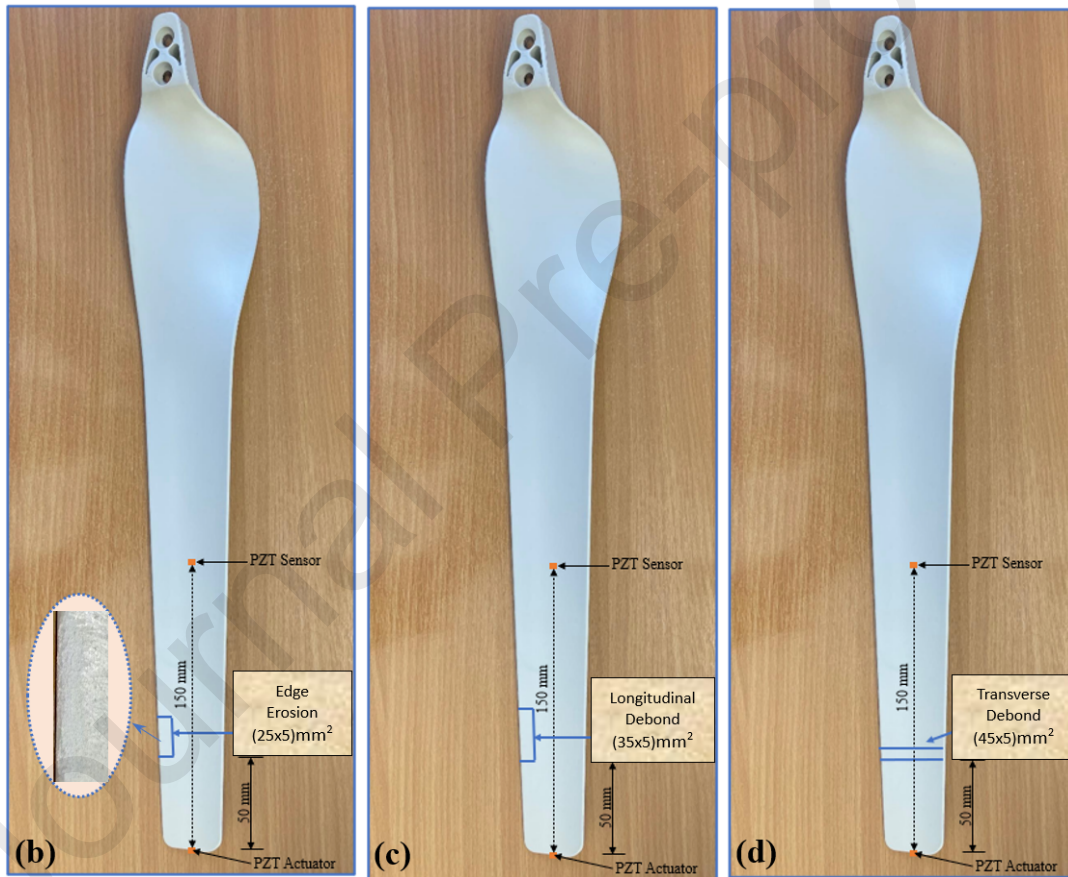
Fig 2. (a) Experimental setup for GW-based inspection of WTB samples, and depiction of WTBs for: (b) erosion damage (c) longitudinal debonding (d) transverse debonding.
