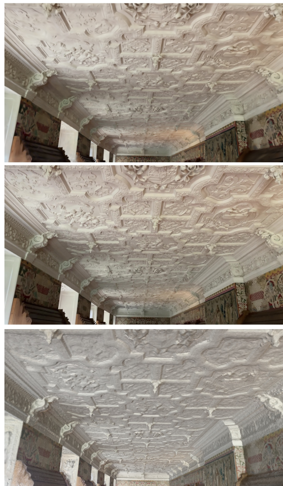
Figure 10: Comparison of 3DGS rendering (top, PSNR: 24.9752 dB, SSIM: 0.7603, LPIPS: 0.5389) and MVS+Poisson meshing (bottom, PSNR: 17.3688 dB, SSIM: 0.4652, LPIPS: 0.6111) against the original evaluation frame (middle).
