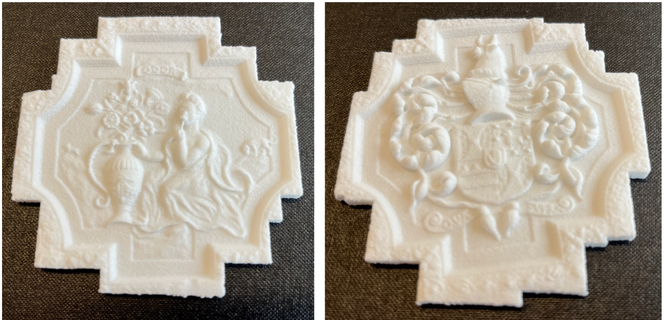
Figure 12: 3D printing prototypes of the scanned 'Odor'(Smell) and 'Arms of Hobart Family' models.
