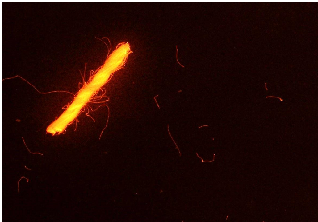
Figure 3.4 Close up image of polyester thread code 23 (as shown in Figure 3.2 and 3.3). The thread can clearly be seen to be fluorescing brighter than individual fibres beside it. Waveguiding of internally reflected photons in individual fibres can also be seen where parts show greater fluorescence intensity. Image brightened by 40 % for display purposes.
