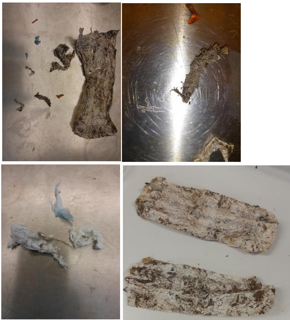
Figure 4.15 Sanitary products and selected macroplastic fragments found in the first cell of the Northrepps ICW
