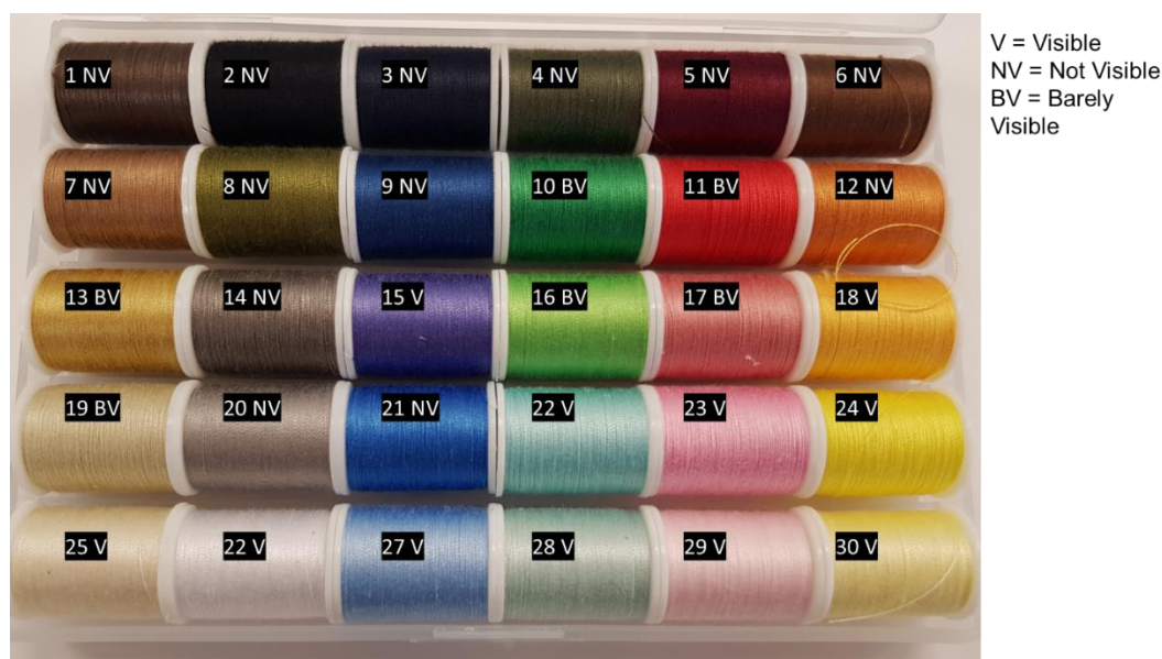
Figure 3.2 Polyester sewing threads that were used to assess Nile Red's ability to stain fibres. Number indicates thread code for correspondence with Figure 3.3
