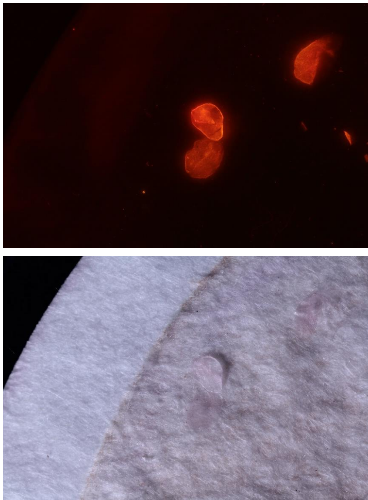
Figure 3.6 Fluorescent (top) and white light (bottom) image of Lemna Minor after digestion with 50 % (v/v) NaClO at 40°C for 16 hours.
