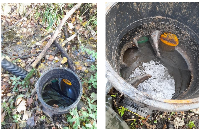
Figure 4.4 Approximately normal flow level in inlet sampling pipe at Northrepps and high flow (right). The main pipe has a diameter of approximately 20 cm.
