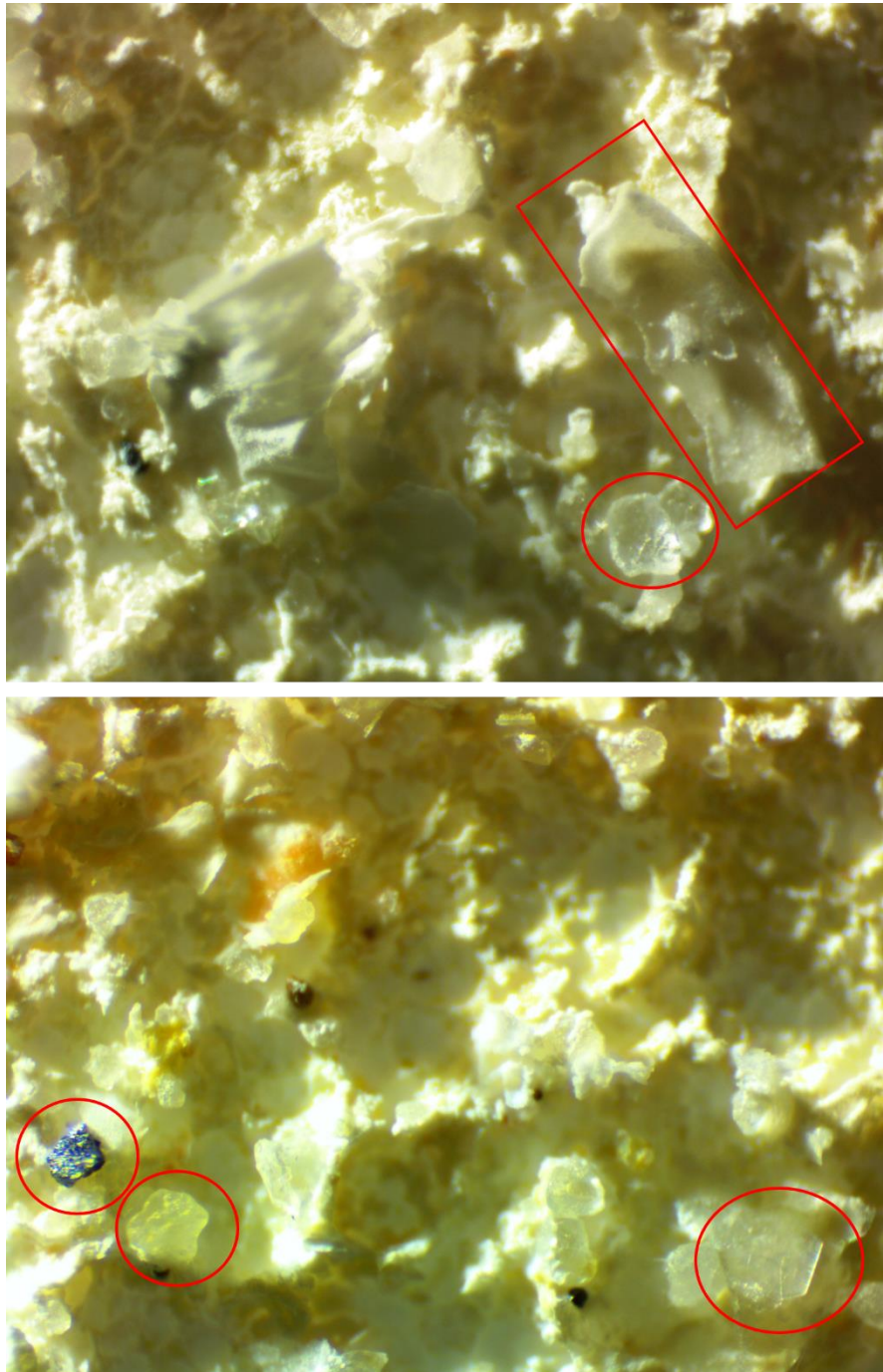
Figure 3.10 Images of a typical sediment sample filter (taken with 4x objective) with potential false positive clear, white and black particles circled.
