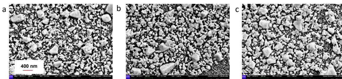
Figure 4.20. SEM images of the film surface of the 10% Ag-Ni/PAA (75:25 w/w%) alloy at different pitch size (a) (45 \mu\text{m} ), (b) (25 \mu\text{m} ), and (c) (15 \mu\text{m} ) at room temperature.
