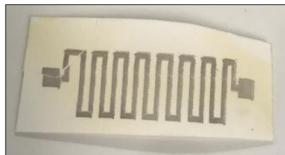
Figure 7.3. Image of a test device on photo paper showing the effect of high temperature on photo paper causing yellowing.
