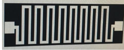
Figure 7.2. Photograph of the temperature sensor design for photo paper.
