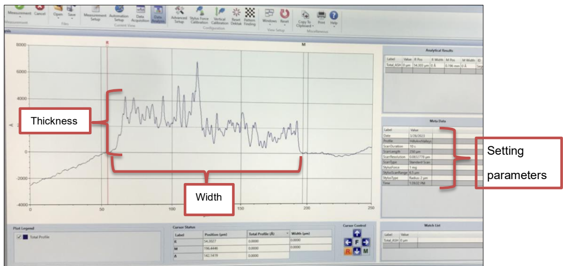
Figure 2.8. Stylus profilometer trace across a printed track.
