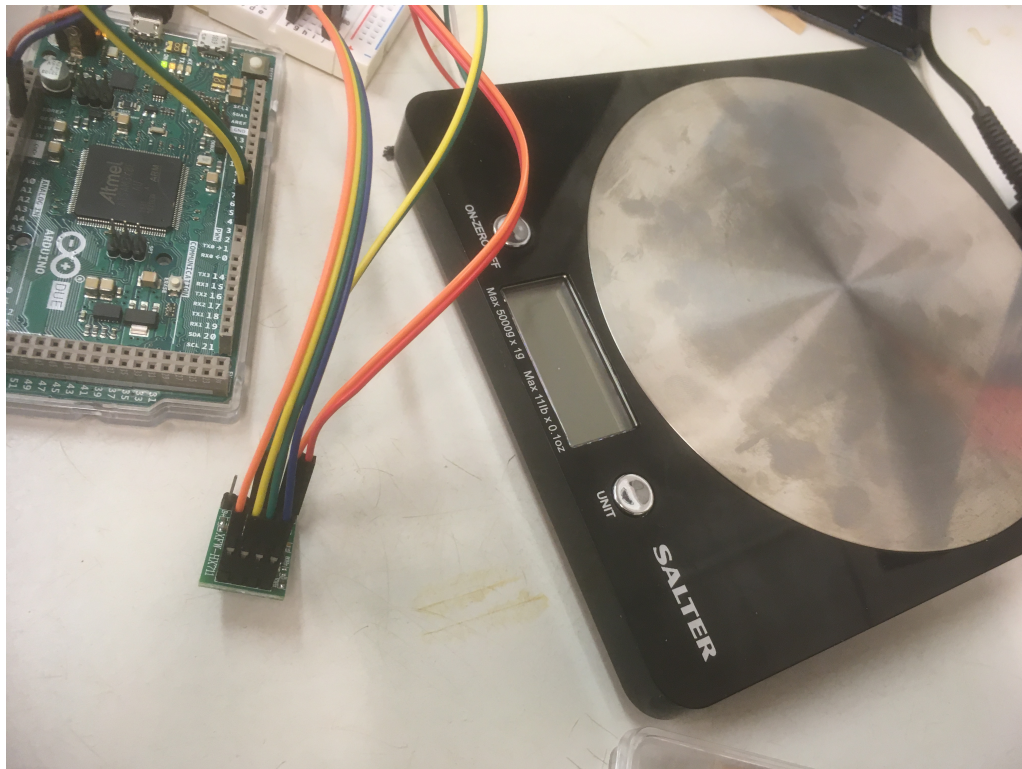
Figure 7.5.3: A hacked pair of scales interfaced with an Arduino to measure extremely low leakage flow.
