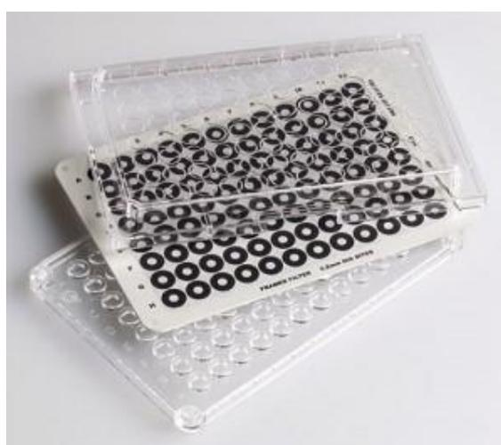
**Figure 2.4 ChemoTX 5  $\mu\text{m}$  pore plate (Neuroprobe Inc, USA).** The plate consists of a 96-well plate where diluted chemokine ligands/vehicle controls were added, a membrane cover where cell suspension were added to allow cells to migrate towards the bottom chemokine-containing wells and a cover (Image source: [https://www.neuroprobe.com/product/chemo\\_tx/](https://www.neuroprobe.com/product/chemo_tx/)).
