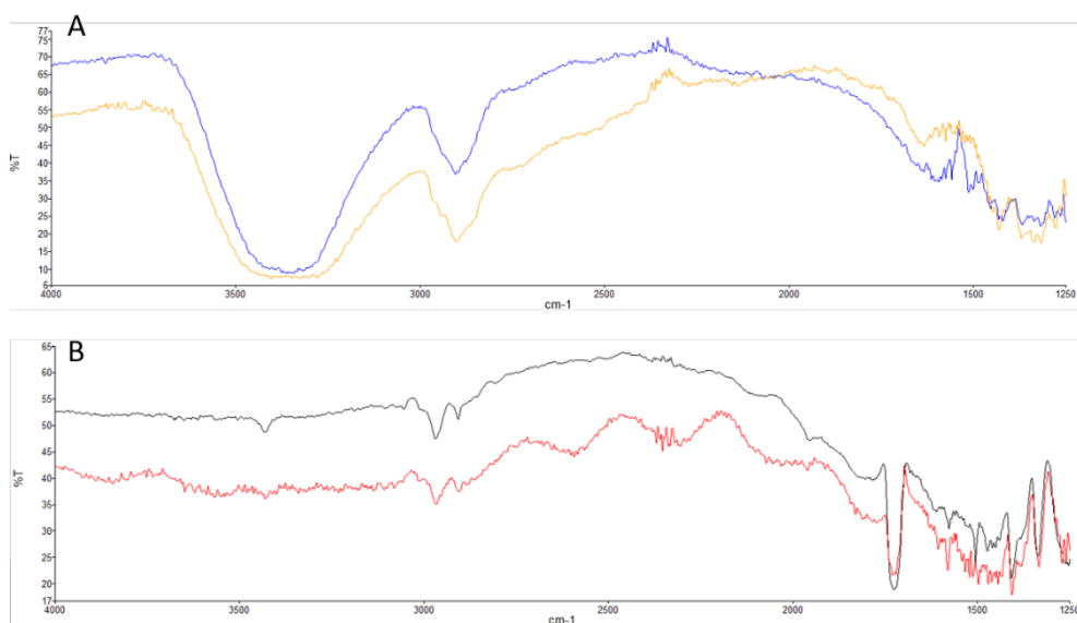
Supplementary figure S13.5. Example experimental microfibre FT-IR spectra pre-exposure and post-exposure (identified within mussel digests). A = cotton microfibrils (yellow = pre-exposure, spectral match = 0.892; blue = post-exposure, spectral match = 0.782), B = Polyester microfibrils (black = pre-exposure, spectral match = 0.897, red = post-exposure, spectral match = 0.673).
