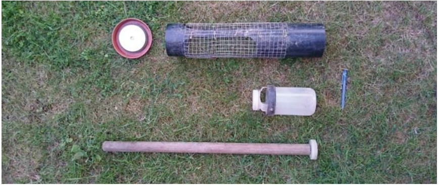
Fig. 1. Components of the old-design hypogean pitfall traps, including push-in top to exclude rain and epigeal species. Dimensions of trap body 50 cm long, 11 cm external diameter. Sample collection port area 500 cm 2 . Sample collection bottle volume 1-L. Note pole with bottle lid attached, used during sample collection.
