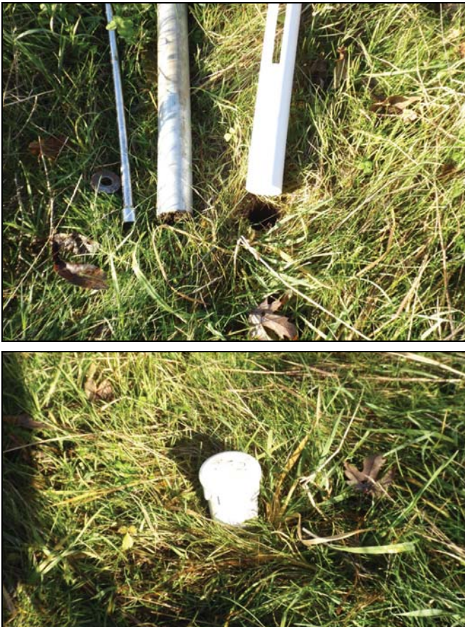
Fig. 5. Top: new-style pitfall trap (right) with corer (centre) and cored hole. Bottom: new-style trap deployed. Note lack of disturbance of surrounding soil.
