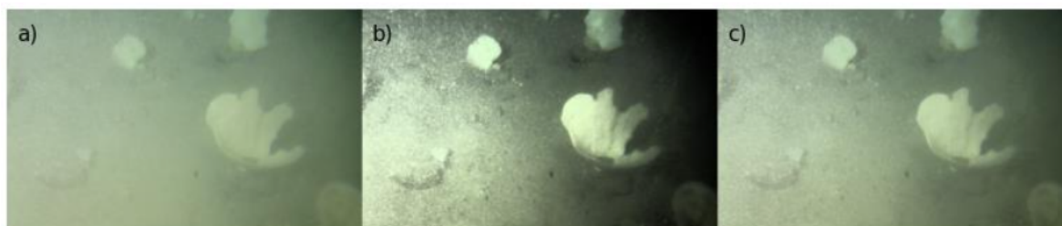
Figure 1: Comparison of an unenhanced image (a) followed by its HE (b) and CLHE (c) tone-mapped output. CLHE min and max slope thresholds were set to 2.56/256 and 0.768/256, respectively.
