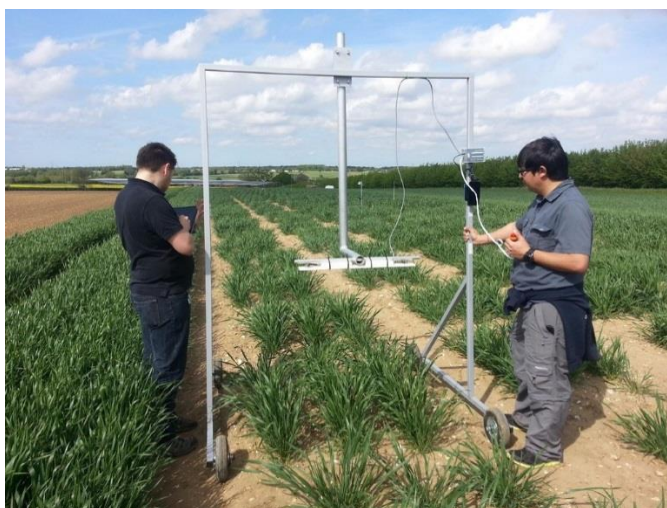
Figure 46. Deployment of the height sensor in Churchfarm Farm, UK. Picture taken 12 May 2015.
