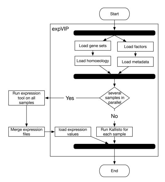
Figure 4.6: The pipeline for loading the data into expVIP. The black lines represent a border of tasks that are not required to be executed in a particular order.
