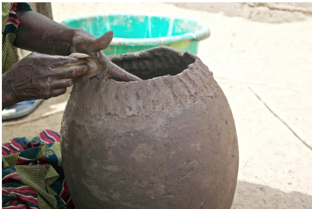
Figure 3.28: Forming of the upper parts of a vessel using hand, mamari, diddinge and makankari.
