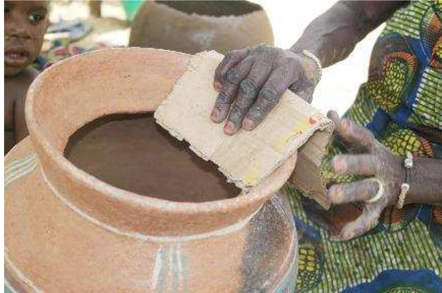
Figure 3.29: Demonstration on how a piece of cardboard is used for refining the rim.
