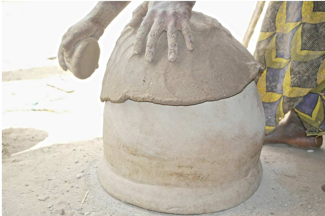
Figure 3.27: Construction of the lower parts of a vessel in Faggo.
