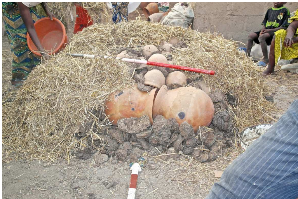
Figure 3.35 : Firing process in Faggo, Shira.
