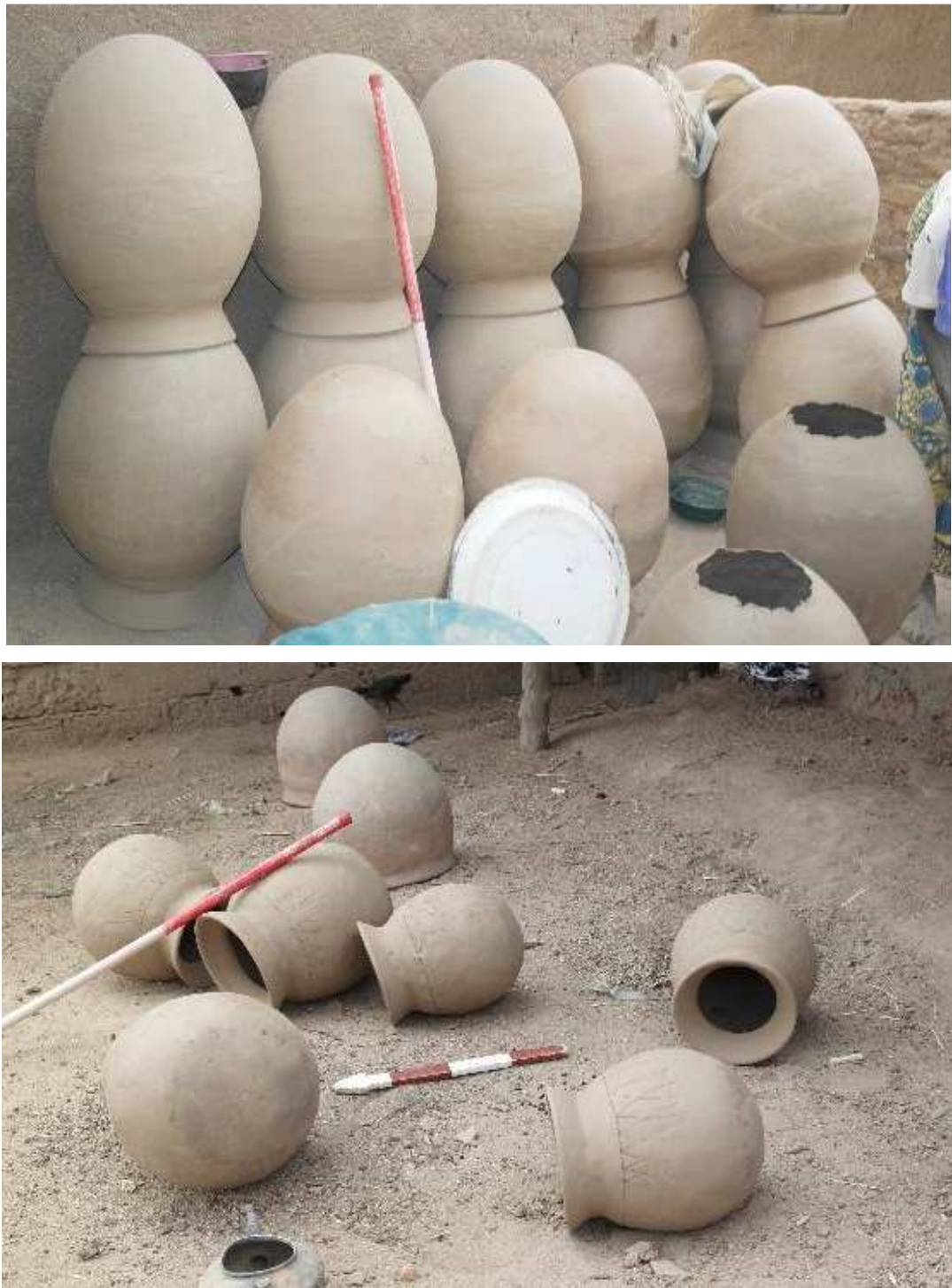
Figure 3.30: Air drying of formed vessels in Faggo and Garande.
