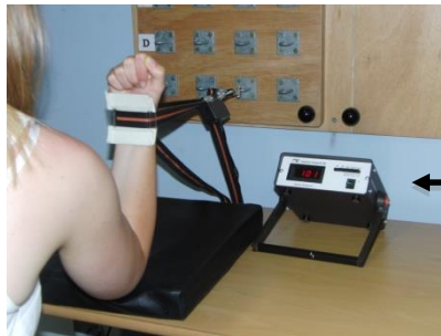
Figure 19 - MTE myometer being used to assess the strength of a biceps contraction.
