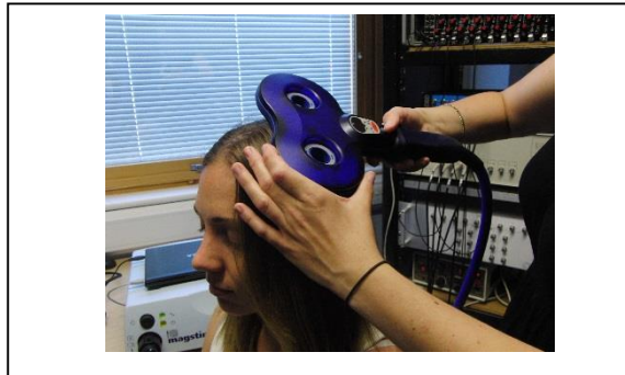
Figure 25 - Coil placement on scalp during TMS collection; tangential to the scalp to obtain a posterior to anterior current flow.
