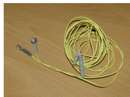
Figure 18D. Cup Electrodes used to collect muscle activity from the APB
