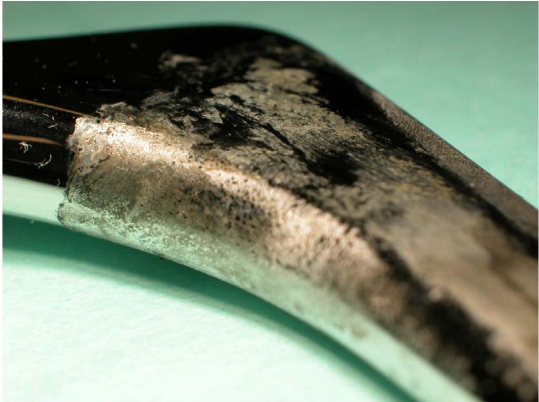
Figure 1.6-11 Ultima TPS femoral stem explant exhibiting characteristic macroscopic corrosion.
