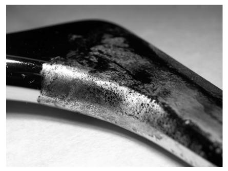
Figure 1-3: Photograph of an explanted Ultima<sup>®</sup> stem. Shows severe corrosion at the interface of the stem and acrylic cement.
