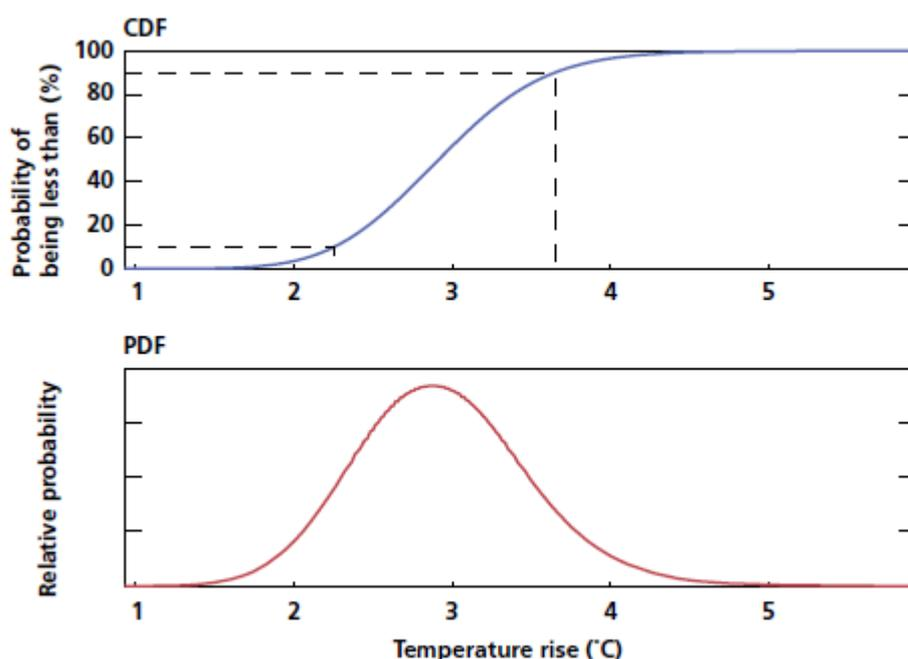
Figure 34. PDFs and CDFs show the same information but in a different form. A PDF can be integrated to form a CDF, and a CDF is a cumulative PDF. A hypothetical example is shown above to show how they relate to each other (Jenkins et al., 2009, fig.8).
