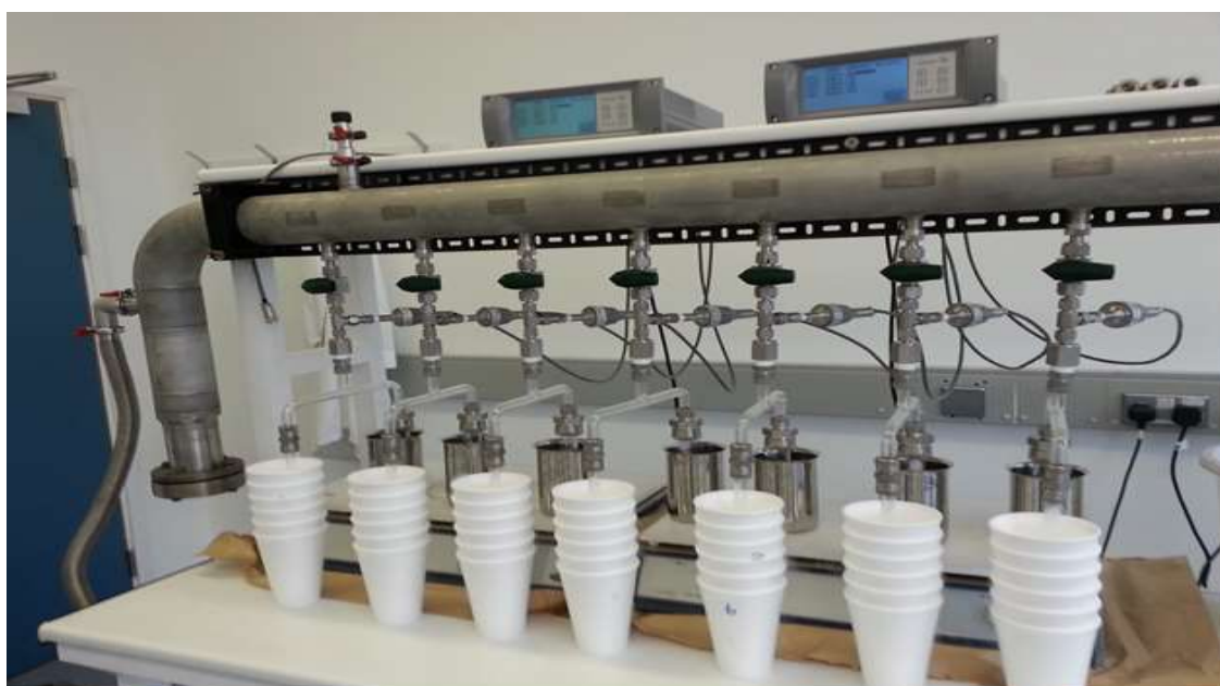
Figure 6.1: cryogenic extraction line at the University of Reading, showing the pressure gauges attached to each station on the line.
