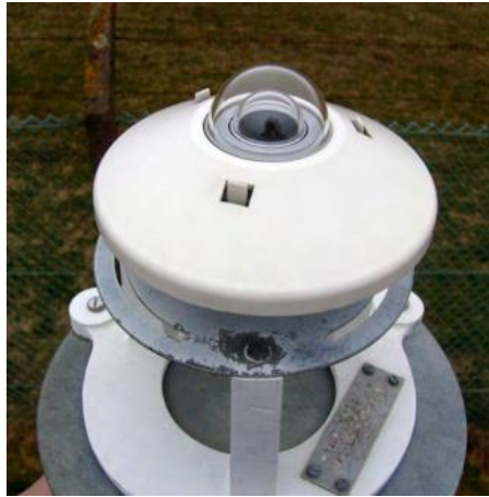
Figure 2.4 Pyranometer for measuring global radiation (MetOffice 2013b)
