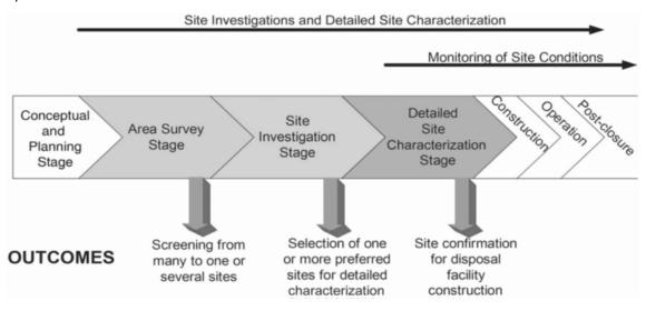
Figure 1: Stages in the development and implementation of geological disposal, with the emphasis on the siting process, IAEA (2011)
