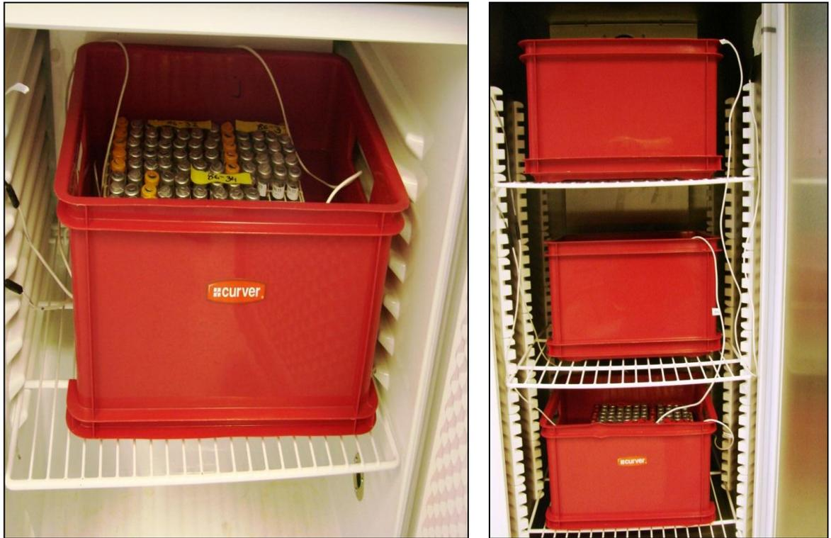
**Figure 3.3** Incubation of inoculated tubes in water-bath, with inserted probes
