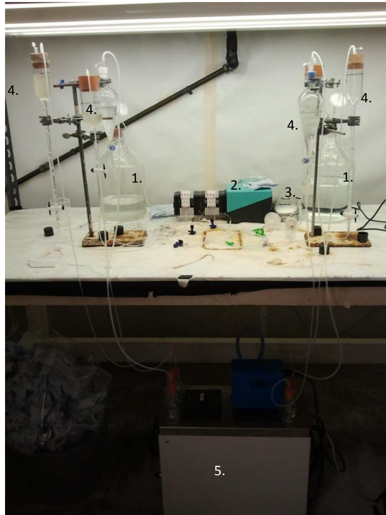
Figure 5-1: Setup of chemostats in the 11°C constant temperature. 1. Medium bottles, 2. Peristaltic pump, 3. Air pump, 4. Culture vessels, 5. Water bath with waste bottles
