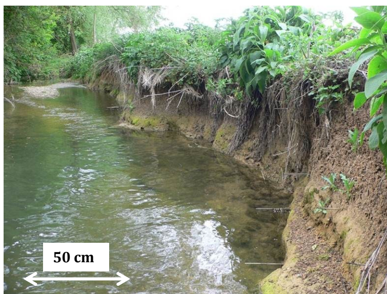
Fig. 2.2.2 Signs of fluvial erosion illustrated by the exposed erosion pins, research site on the River Stour in East Anglia (Fig. 1.1.1), May 2009.
