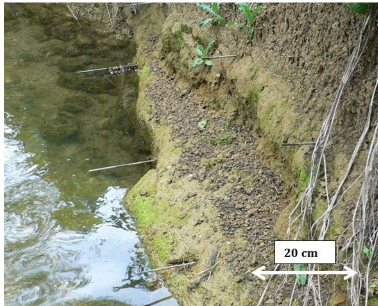
Fig. 3.4.1 Detail of erosion pins on field site LB1 in Little Bradley (see location map on Fig. 3.1.1). The flat piece of bank is possibly indicating the level of a prolonged water transfer. Erosion pins show retreat that occurred between June 2007 and May 2009 (see also Fig. 3.5.1).
