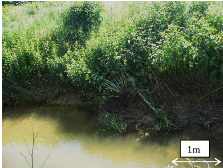
Fig. 3.4.26 Slumped piece of the right bank at GB1 site (Fig. 3.1.1) with the uprooted tall herbal vegetation, June 2007. Failed material is covering the lower pin.
