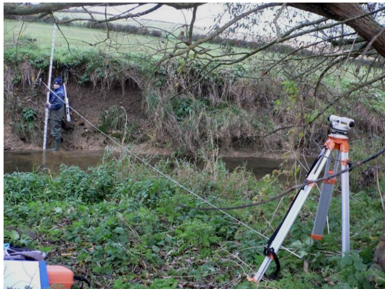
Fig. 3.4.3 Channel cross section surveying using Nikon automatic level at GB2 site in Great Bradley.
