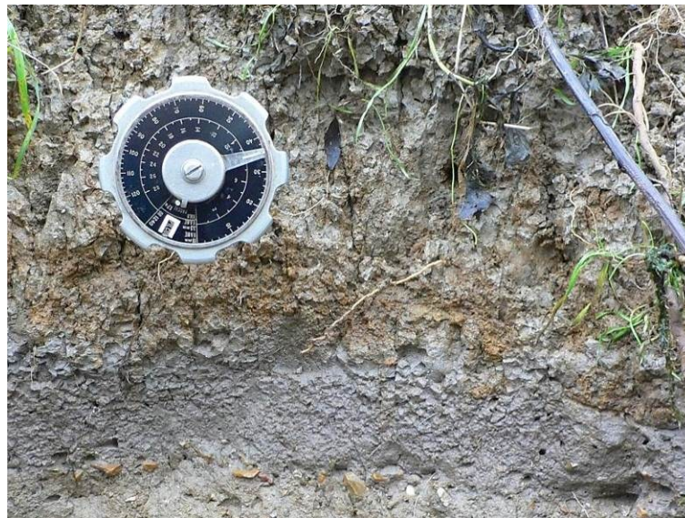
Fig. 3.2.12 In situ soil shear strength testing using the Field Vane at the S1 site (Fig. 3.1.1). Sedimentary layers with material of different texture are distinctive in the bank, mainly the grey lens of clay below more sandy and silty material.
