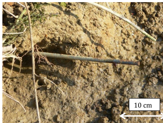
Fig. 3.4.27 A large cavity formed around the pin LB1-3B. Left bank at LB1 site near Little Bradley, January 2008 (Fig. 3.1.1).
