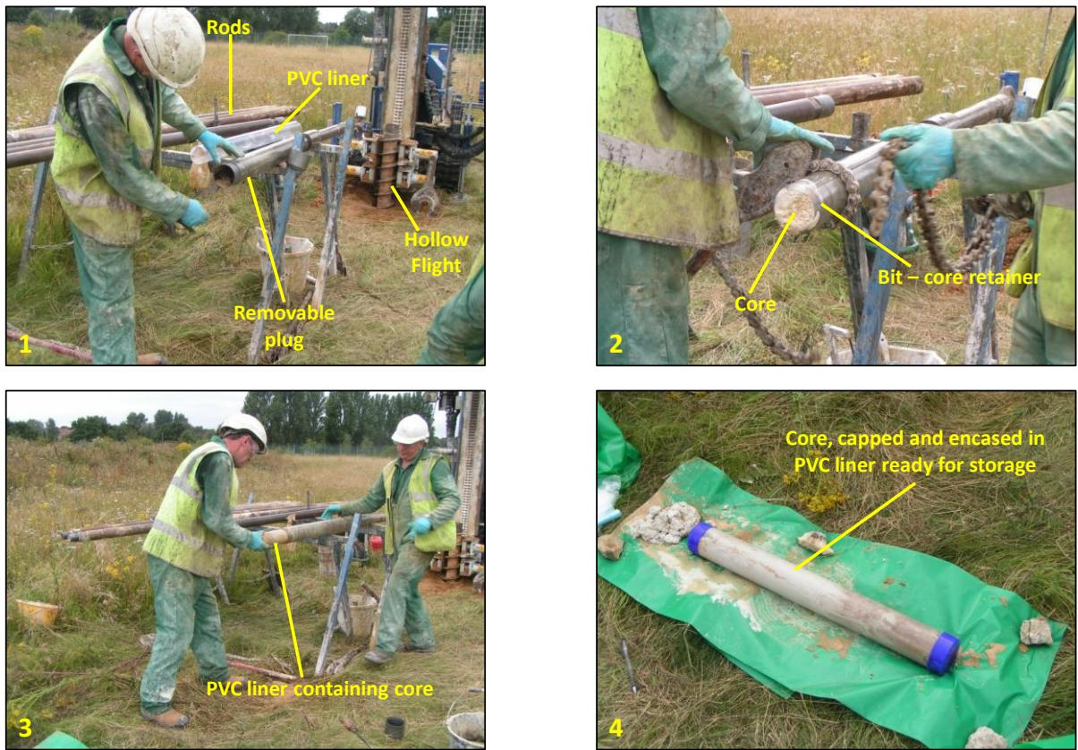
**Figure 5.2.4 - Collection of core sample.** 1) The plug was loaded with a PVC liner and inserted into the hollow flight with the aid of rods. 2) At 1 m intervals, the rods were removed and the core recovered from the plug. 3) The bit was unscrewed and the PVC liner, containing the core, removed from the plug. 4) The PVC liner was capped, sealed and the core placed in cold storage.
