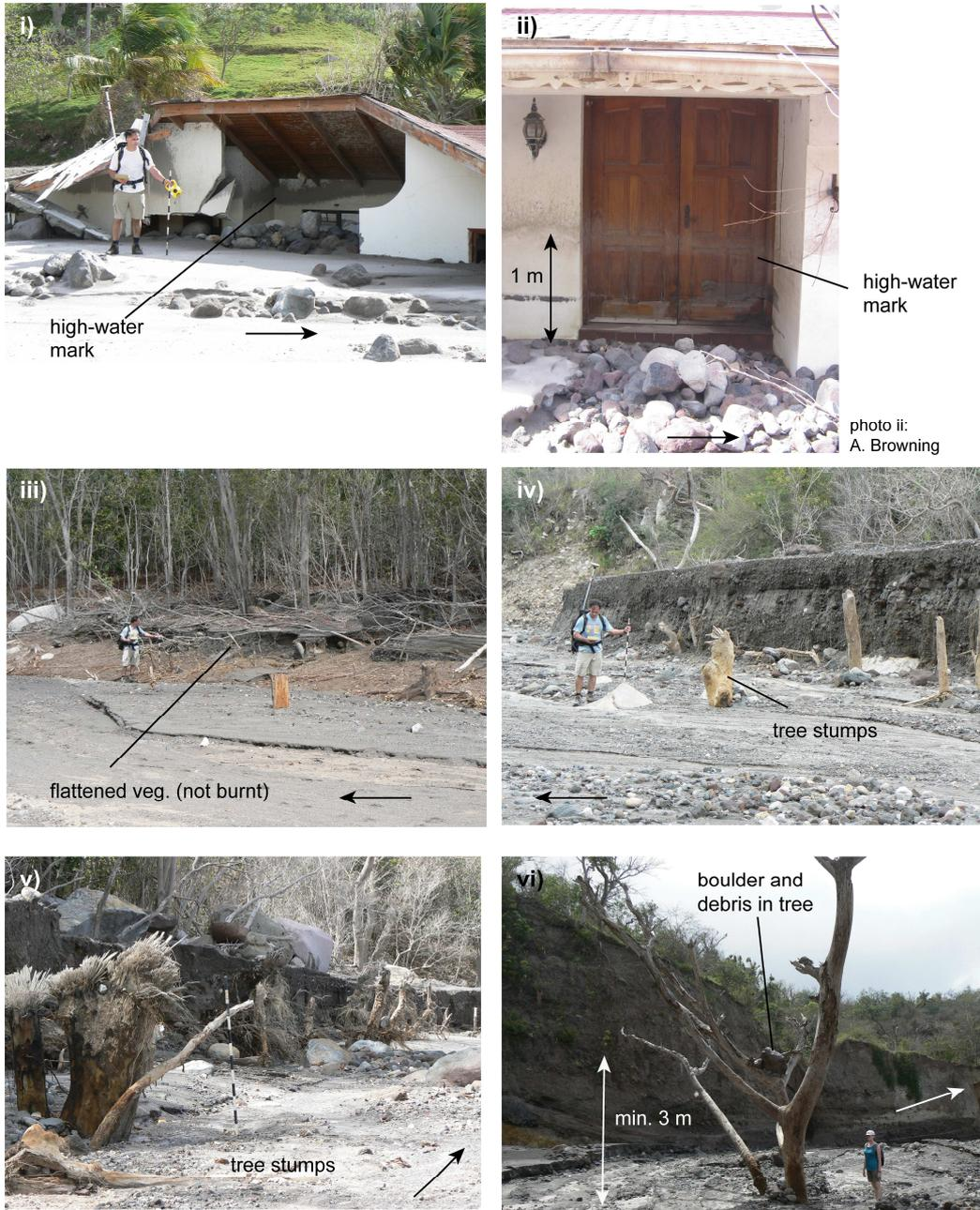
**Figure 5.4** Stage (flow height) indicators included damaged vegetation, stranded boulders and high-water marks. These photographs progress in sequence from the lower-reach (i and ii) to mid-reach (iii) to upper-reach (iv, v and vi); arrows represent flow directions. A measuring stick with 0.1 m divisions was used for scale.
