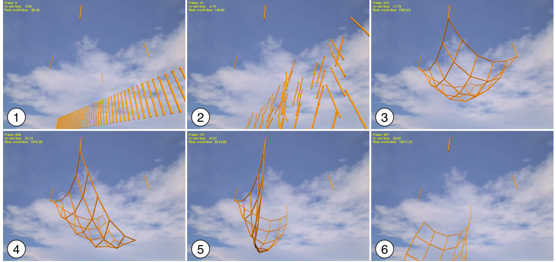
Figure 3.2: Implementation by thesis author of Barzel and Barr’s dynamic constraint modelling system. The rigid bodies (1) fly together (2) and self-assemble into a structure (3) hanging from four point-to-nail constraints, while swinging naturally, as described in [BB88]. The realistic swinging and waves rippling within the chain mail-like structure continue, as it is gradually released (4,5) and falls away (6). The four static segments serve to highlight the point-to-nail constraint locations.
