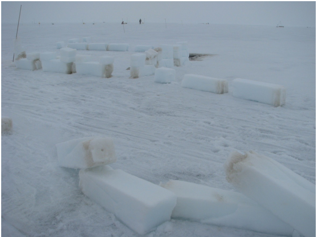
Figure 86. Large pieces of sea ice cut to make holes for the dive team. Large volumes of brine were collected from these \sim 0.25\text{m}^3 pieces of brine for incubation studies, however as is clear from the photograph, the diatom colonies did not drain from the ice with the brine.
