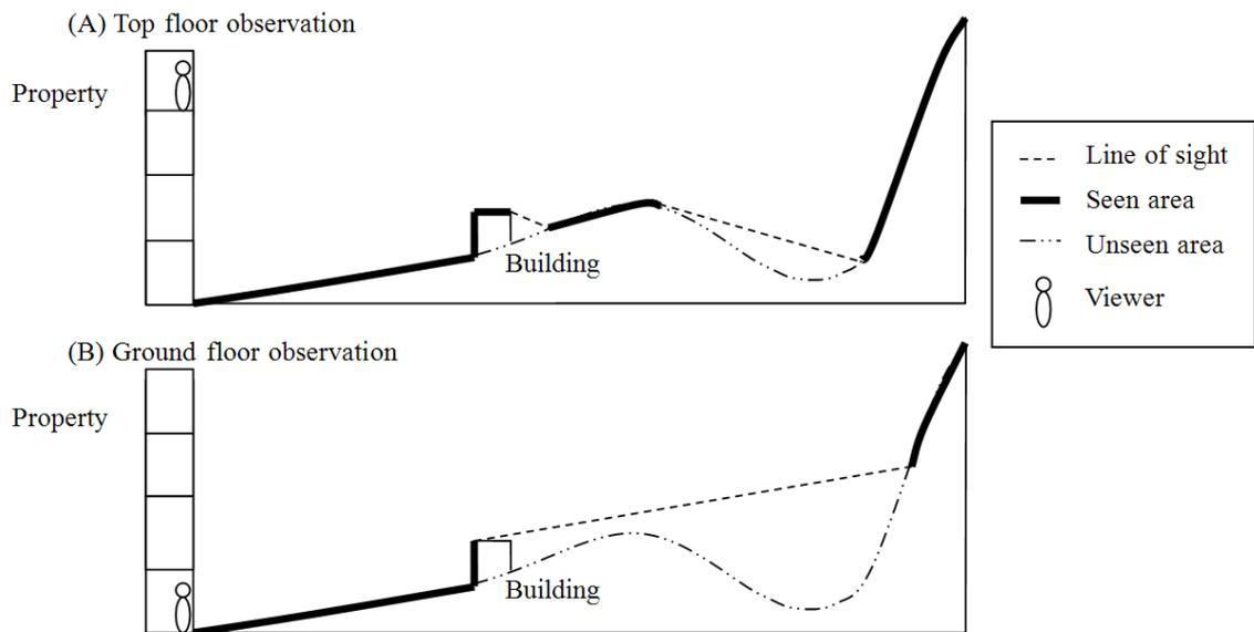
Figure 6.3. The computation of visibility from the ground and top floor
