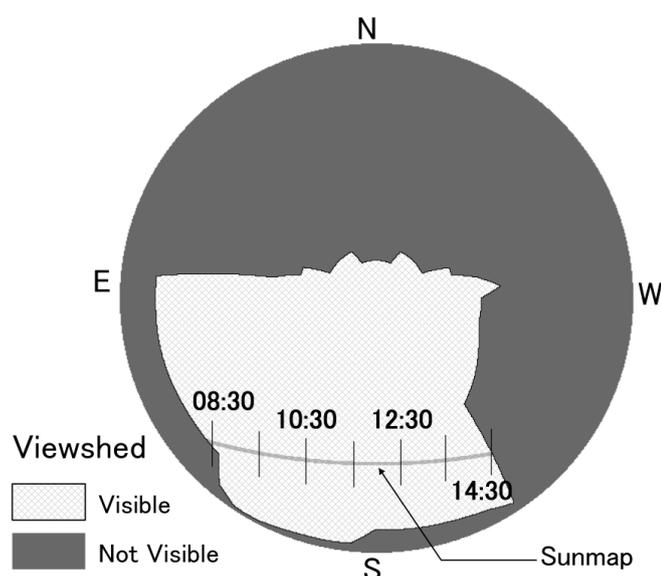
Figure 5.5. The calculation of sunshine duration on a sample calculation point on the winter solstice 2000
