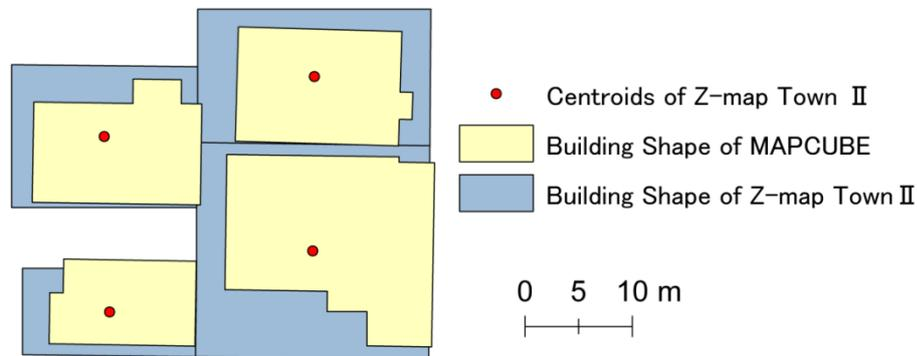
Figure 5.3. The method used to combine the two building datasets
