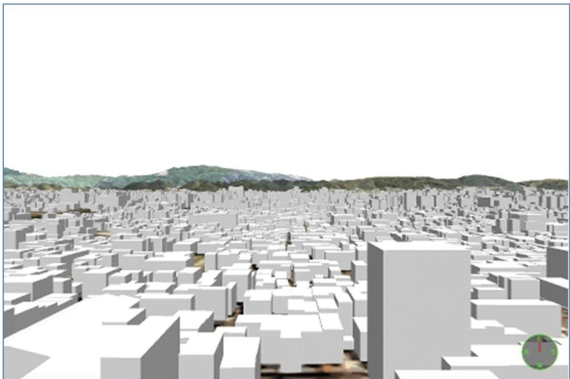
Figure 5.2. Building shape polygons from MAPCUBE
