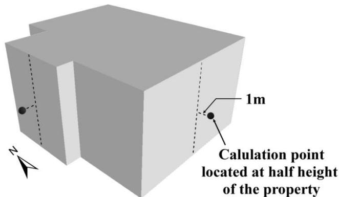
Figure 5.4. The location of calculation points on buildings
