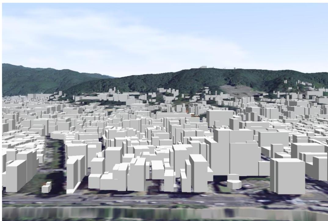
Figure 6.2. Example building shape polygons derived from MAPCUBE data
