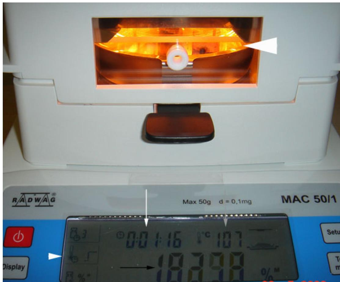
Figure 5.2 Hydration analyser during the drying process. The heating element raises the temperature in the drying chamber (white arrowhead); the temperature within the drying chamber is displayed on the LCD screen (grey arrow) together with the elapsed time (white arrow), mass reading (black arrow) and the cycle setting (white arrowhead).
