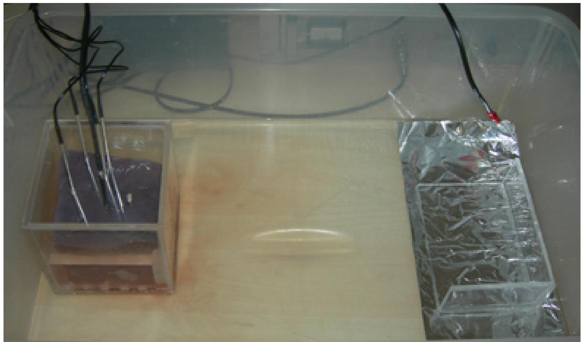
Figure 2.4 Perspex box containing piece of liver with electrode (black rod), temperature probes (silver rods) in situ. Foil grounding pad placed 20cm from the liver.
