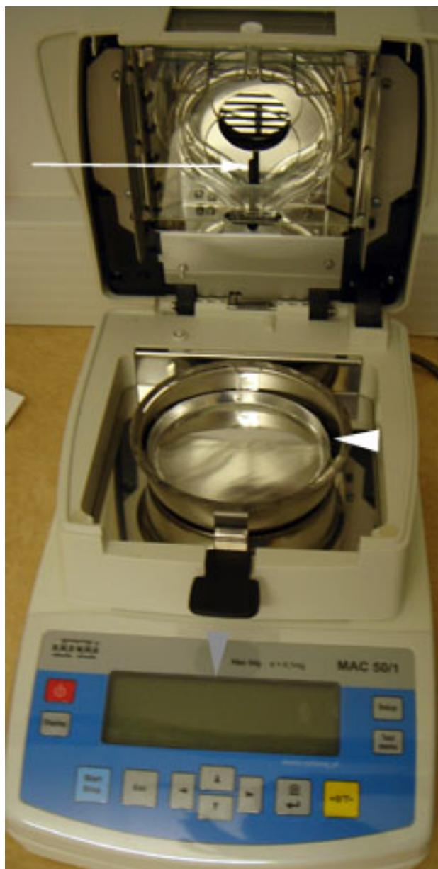
Figure 5.1 the Radwag MAC 50/1. Heating element (white arrow), disposable tray (white arrowhead) and LCD display (grey arrowhead)
