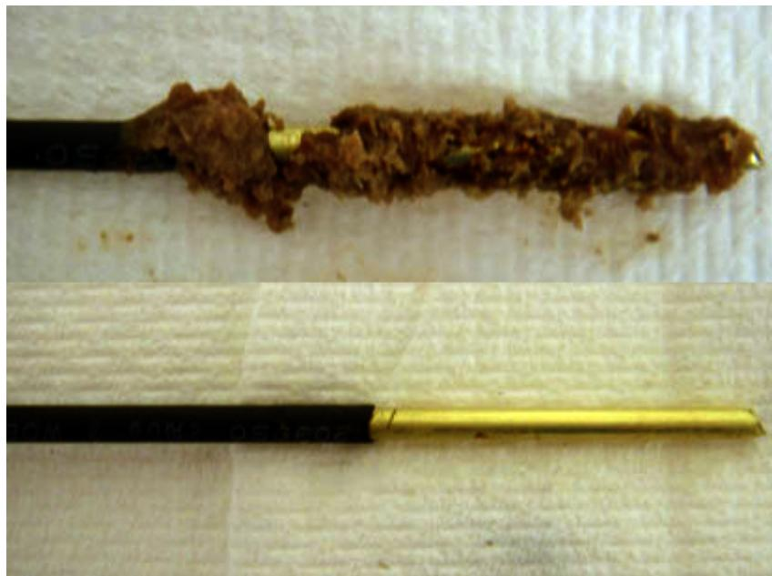
Figure 2.8 charred adherent tissue following conventional RFA (top) and the appearance of the needle following BETA (bottom)
