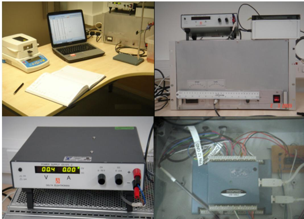
Figure 1.5 Clockwise from top left, laboratory set-up, BETA Mark II machine, DC supply, and digital/analog convertor.
