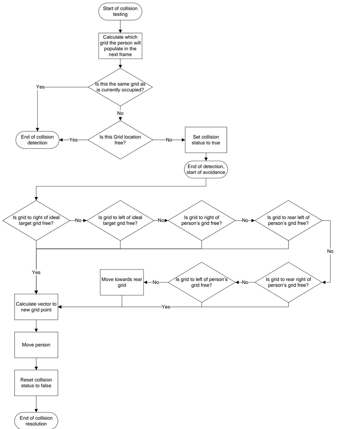
Figure 12. Flowchart of the grid collision detection and resolution method.
