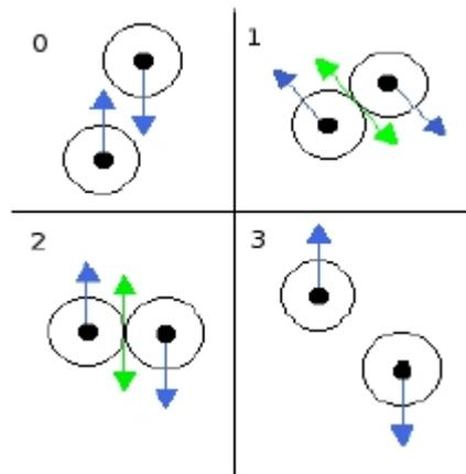
Figure 9. The stages of collision avoidance, showing agents shearing past one another. Adapted from [Champagne, 2005].
