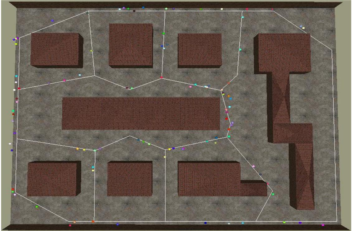
Figure 25. The final implementation showing agents (represented by spheres) following the paths created by the Voronoi Graph method.
