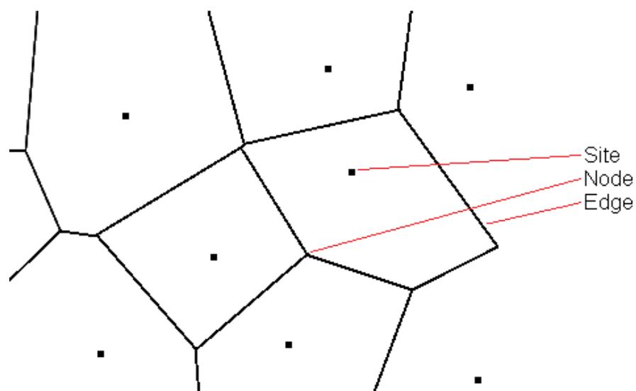
Figure 5. Voronoi diagram. Displaying Sites as the points from which a Voronoi graph is calculated, Nodes as the intersections between Voronoi regions, and Edges as the boundaries of these regions.
