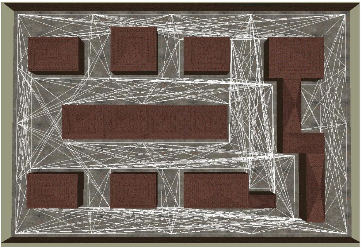
Figure 18. Lines rendered between points in the Visibility Matrix show all possible path routes that can be chosen by an agent when moving from goal to goal.
