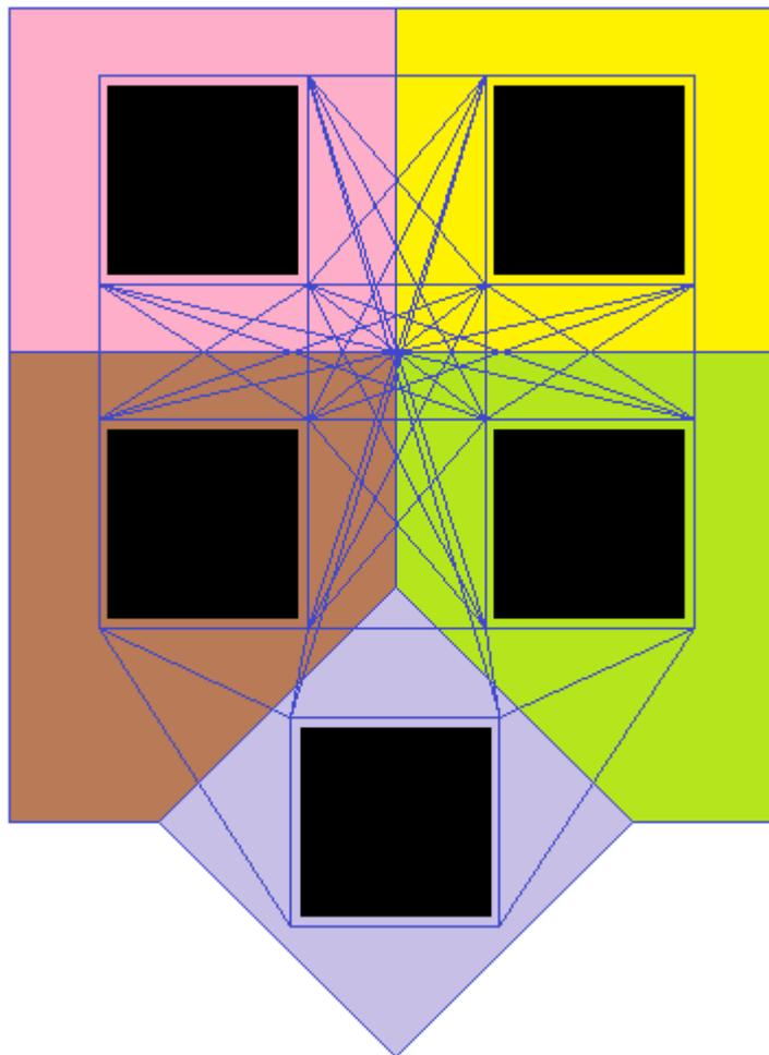
Figure 27. Using a Voronoi Graph to subdivide a given scene that already contains waypoints for agent navigation.
