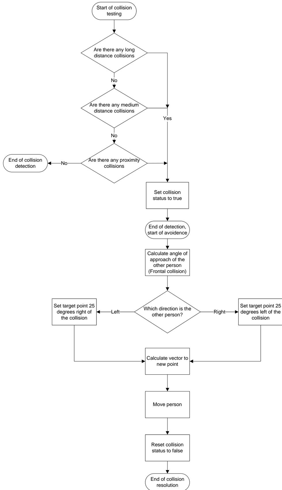
Figure 11. Flowchart of the Proximity collision detection and resolution method.
