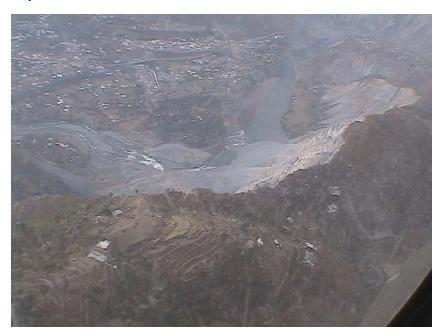
Figure 4.40: Agricultural terraces disturbed above the Chela Bandi landslide of Figure 4.5
