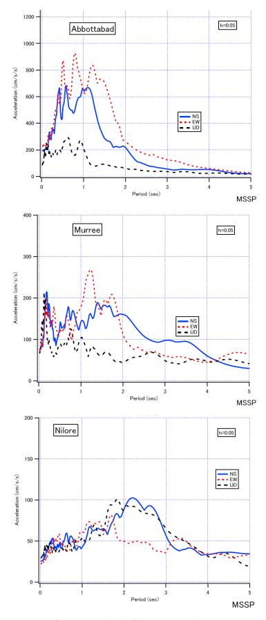
Figure 2.11: Response spectra of ground motions (5% damped, elastic) recorded at Abbottabad, Murree and Nilore (Chaudury, 2006)
