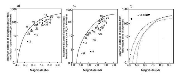
Figure 4.1: Relationships between maximum distance of landslides from causative fault and earthquake surface wave magnitude: a) disrupted slides and falls, b) coherent slides, c) envelopes to a) and b) and lateral spreads (dotted line) (after Keefer, 1984)
