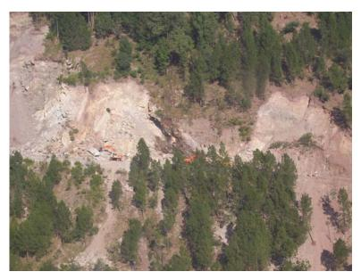
Figure 4.23: Shallow depth landslide exposing the underlying rock. Mixture of rock fall and soil flow block the northern access road to Balakot City, NWFP (photo by Kathrin Renner (Arup) and US Army)
