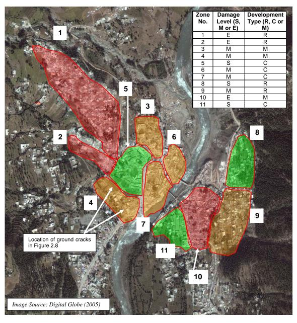
Figure 3.10: Selected damaged areas in Balakot city
