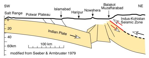
Figure 2.5: Cross-sectional view of the rupture area in the Indus-Kohistan Seismic Zone
