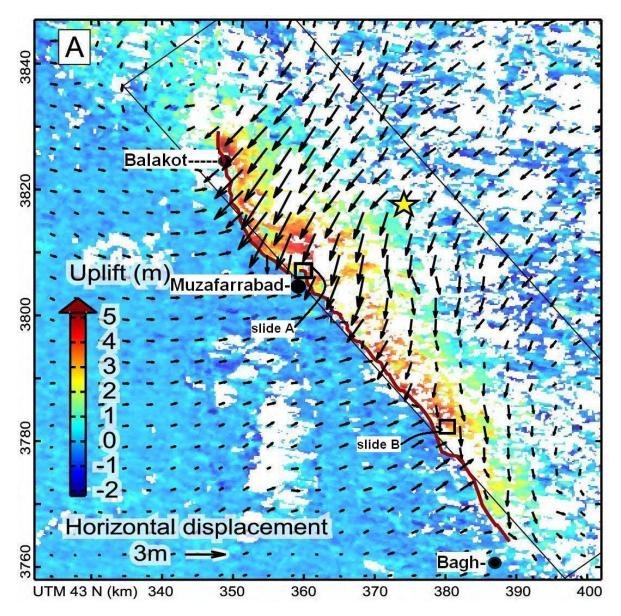
Figure 4.2: Displacement of the Earth's crust caused by the Kashmir 2005 earthquake. Black arrows indicate horizontal displacement and colour vertical uplift, the star indicates the epicentre (adapted from Pathier *et al.*, 2006). Significant landslides discussed in the text occurred at "slide A" (Muzafarrabad slide) and at "slide B" (Hattian slide)
