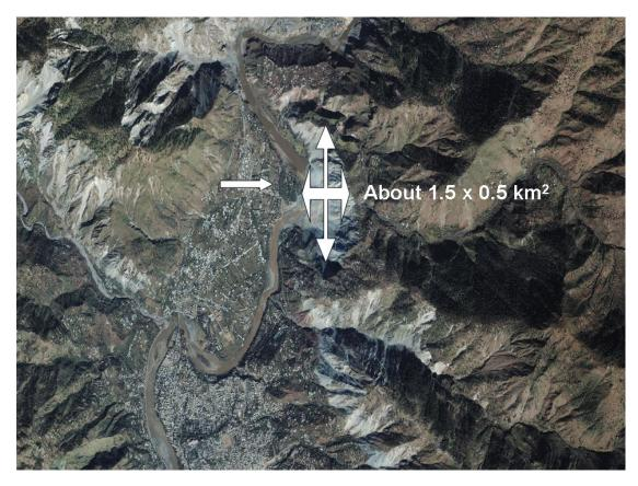
Figure 4.6: Main landslide at Chela Bandi, north of Muzafarrabad, imaged from space (Image NASA) with extent 1.5 km N-S and 0.5 km E-W. Arrow to the left indicates point of view in photographs of Figures 4.4 and 4.5
