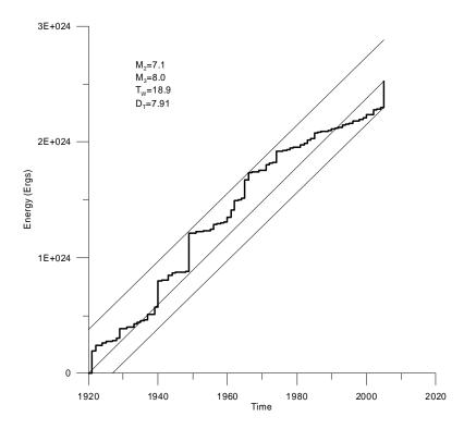
Figure 2.16: Cumulative Strain Energy Release (CSER) for non-probabilistic modelling of seismicity and estimation of maximum credible earthquake in a region. The region occupies 10° of latitude and longitude centred on the Kashmir 2005 earthquake epicentre: a) excludes the Kashmir earthquake and b) includes the Kashmir earthquake as the last step in the energy release staircase (after Burton and Cole, 2006)
