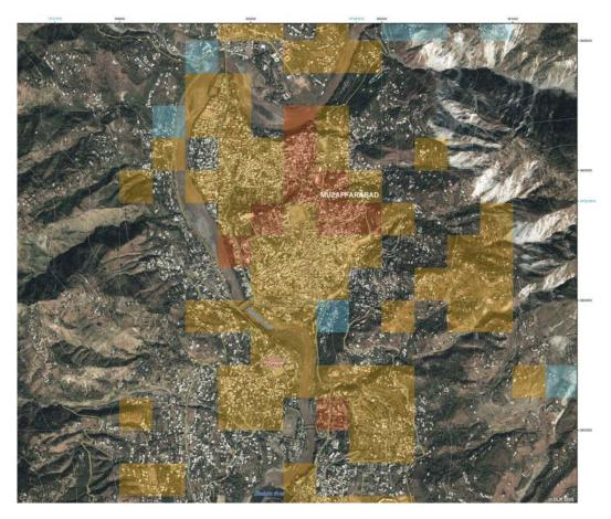
Figure 3.19: Satellite image of Muzaffarabad city centre after the earthquake with spatial damage levels (UNOSAT, 2005)
