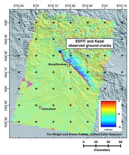
Figure 2.6: Map showing the location of the causative fault of the October 8, 2005 earthquake (Source: COMET, 2005)
