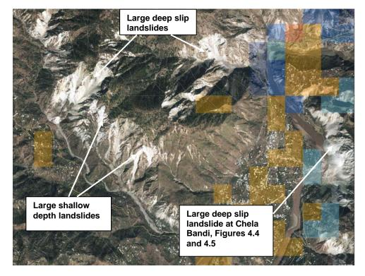
Figure 4.11: Landslides in the northern part of Muzaffarabad City, AJK (UNOSAT, 2005)
