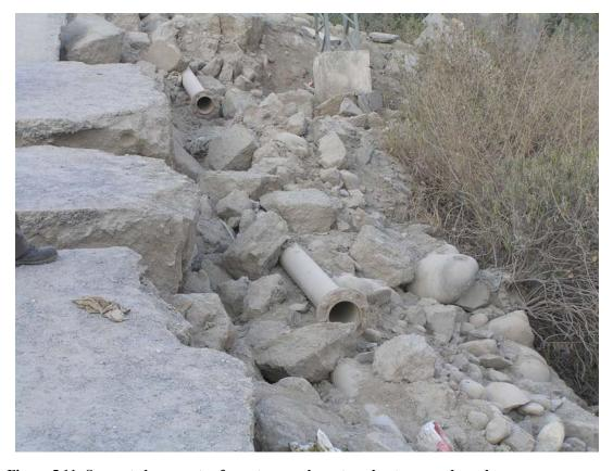
Figure 5.11: Separated segments of a water supply system due to ground cracks, Muzaffarabad
