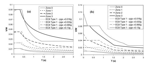
Figure 6.3: Examples of the plots of normalized base shear vs building fundamental period given by the Pakistan 1986 Seismic Code and Eurocode (EC) 8 used to find the PGA corresponding to each seismic zone: (a) Normal importance, non-ductile frame and rock-site conditions, (b) Normal importance, ductile frame and soil conditions
