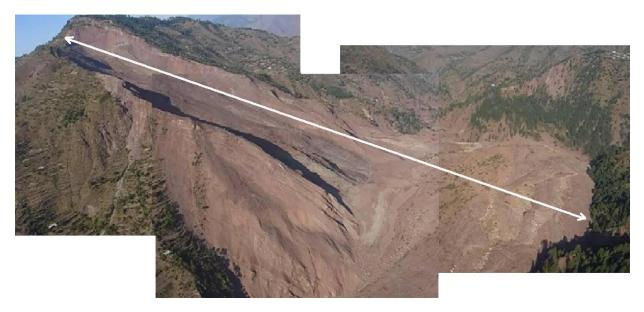
Figure 4.9: The Hattian slide, Pir Punjal Mountains: the major landslide in the Kashmir 2005 earthquake. This deep cutting landslide from source scarp to toe (white arrow) stretches over approximately 2,850 m (photo collage by Charles Scawthorn)
