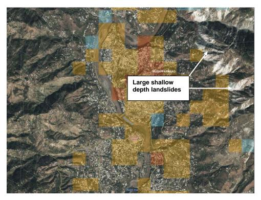
Figure 4.12: Landslides in the central part of Muzaffarabad City, AJK (UNOSAT, 2005)
