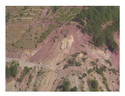
Figure 4.22: Shallow depth landslide and slumping of soils blocking an access road to Balakot City, NWFP (photo by Kathrin Renner (Arup) and US Army)
