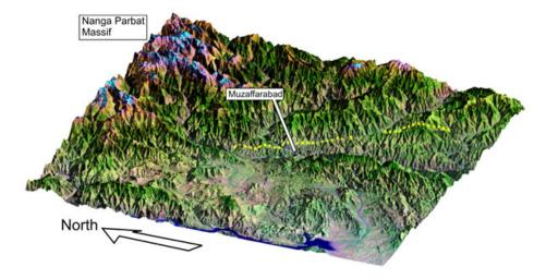
Figure 2.7: 3D perspective view of the Kashmir earthquake region and Muzaffarabad. The image is formed by draping LANDSAT 7 imagery over NASA SRTM (Shuttle Radar Topography Mission) digital topography. The fault identified by radar imagery is marked as a yellow dotted line. The mountains are higher on the far (north-eastern) side of the fault. (Source: COMET, 2005)
