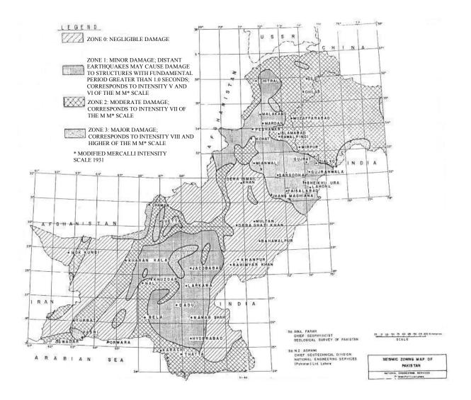
Figure 6.1: The Pakistan seismic zoning map (as per 1986 Pakistan Seismic Code)
