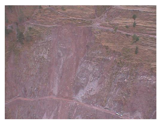
Figure 4.43: Agricultural terraces slipping down steep terrain and valley-side road, all threatened by landslide, near Dhanni Nelam (Dhanni Nelam-Islamabad flight)
