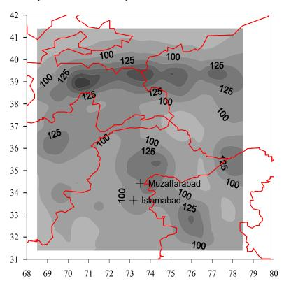
Figure 2.14: Ground shaking seismic hazard map for Kashmir using Sharma's (1998) attenuation law. The contours are expected maximum peak ground accelerations in cm s<sup>-2</sup> with a one-in-ten chance of being exceeded during 50-years (extracted from Burton and Cole, 2006)
