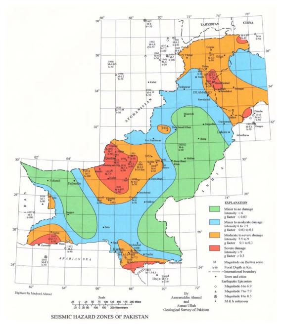
Figure 2.13: Seismic hazard zoning map of Pakistan issued by Geological Survey of Pakistan (after Ahmed et al., 2006)
