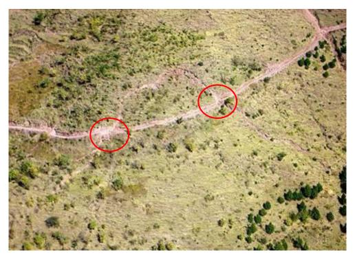
Figure 4.36: Incipient landslide threat to road: the road is cut in two places by cracking (photo by Charles Scawthorn)
