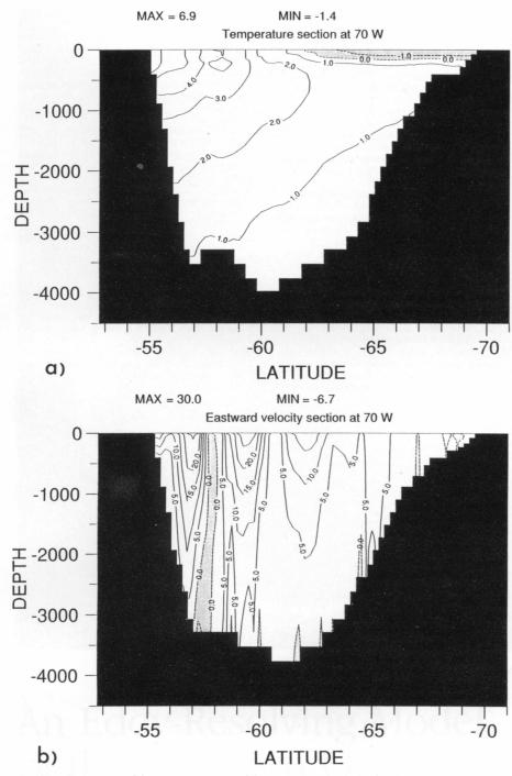
Fig. 3. Contours of (a) temperature and (b) eastward velocity on a north-south section across the Drake Passage at 70°W at the end of 6 years. Contour intervals: (a)  $1^{\circ}$ C, (b) 0.05 ms<sup>-1</sup>. Negative values shaded.
