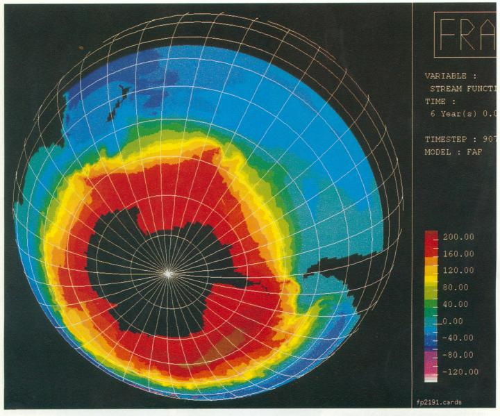
Fig. 1. Contours of stream function (depth integrated transport) in units of  $10^6 \text{m}^3 \text{s}^{-1}$  at the end of 6 years.
