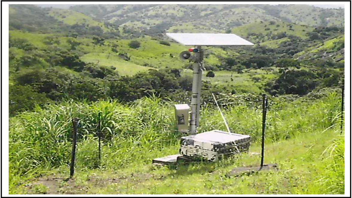
Figure 8.6: Carbon-dioxide gas detector and sound warning system placed in Lake Nyos. Source: Author (picture taken during fieldwork in Cameroon in 2007)
