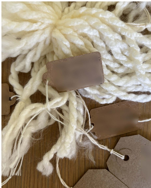
Fig 15. LTA threads tied, frayed, broken (image f).
