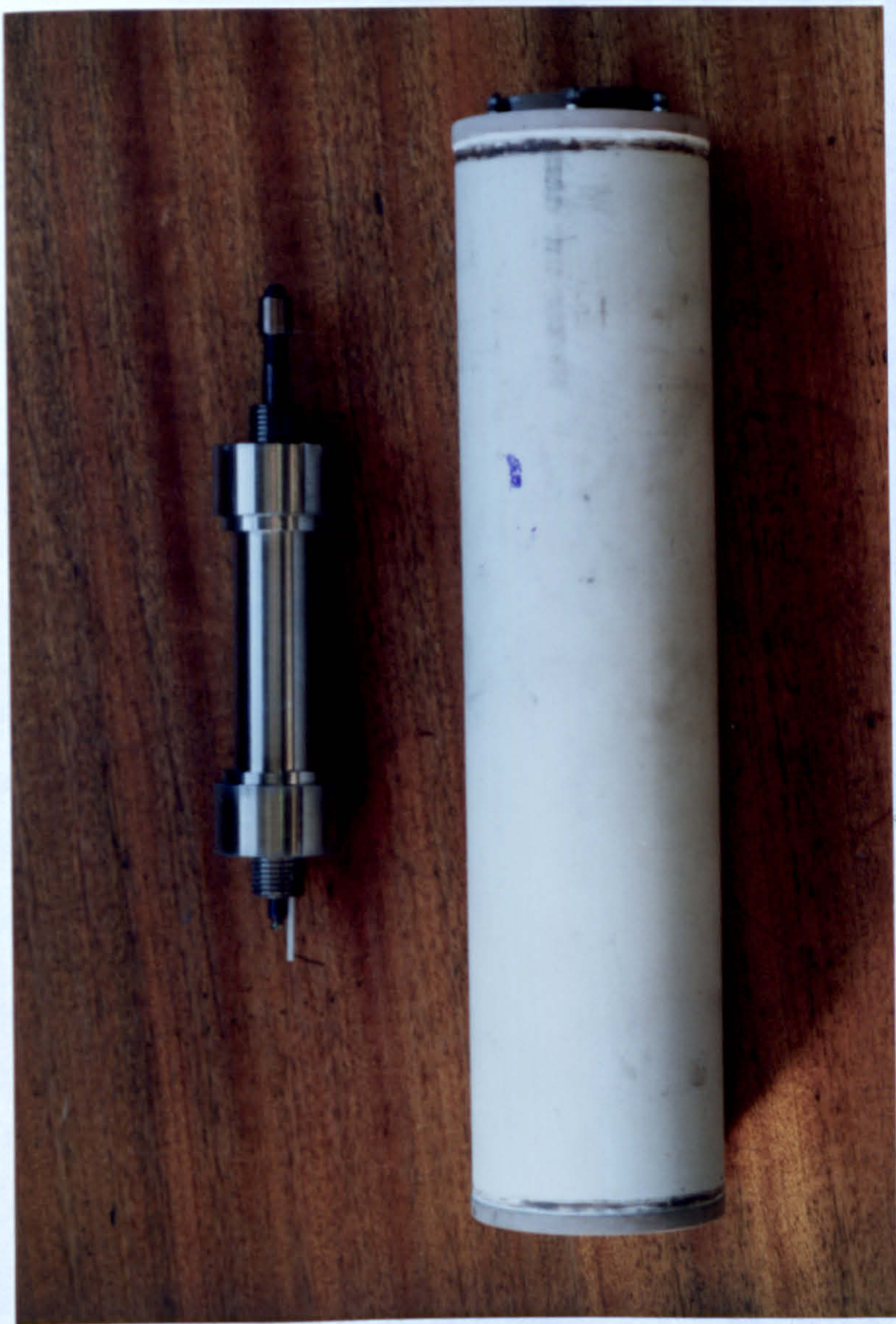
PLATE P5.3. THE FURNACE AND A FULLY PREPARED EXPERIMENTAL CELL
