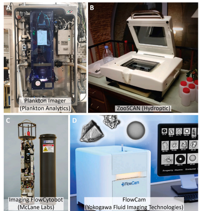
Fig. 3. Four examples of instruments currently used for automated imaging methods in plankton monitoring. The Plankton Imager (A) (Pi-10; Plankton Analytics), consists of a high-speed camera that images all passing particles in a flow of pumped seawater. Images are identified in real-time and uploaded via satellite. The ZooSCAN (B) (Hydroptic) uses a flatbed scanner with specialised lighting and a watertight scanning chamber to record high-resolution images of zooplankton samples. The Imaging FlowCytobot (C) (McLane Labs) is an automated submersible imaging flow cytometer that captures high-resolution images of a single-file flow of particles (triggered by fluorescence) in situ . FlowCam (D) is a flow imaging microscope that captures high-resolution images of microscopic particles as they pass through a flow chamber.
