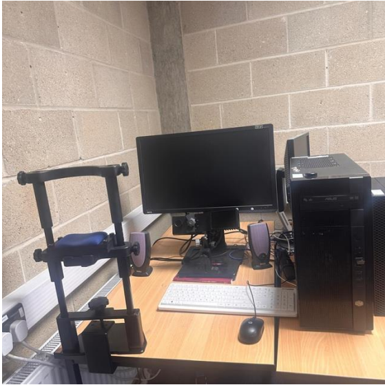
Figure 28 Showing EyeLink 1000 Plus to capture eye tracking data as stimuli is displayed on the screen and set up in actual lab used for the current study
