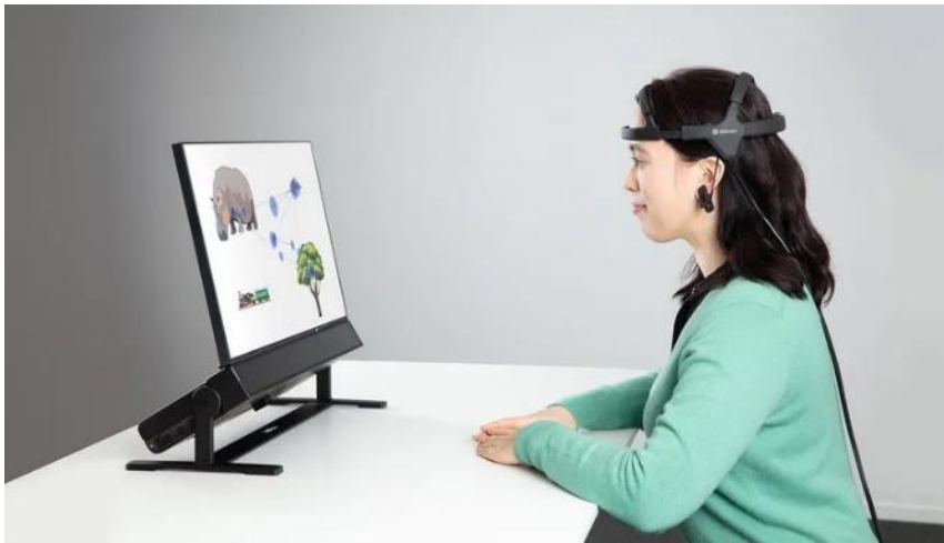
Figure 20 The image shows an eye tracker worn by a participant for a desktop eye tracking exercise.
