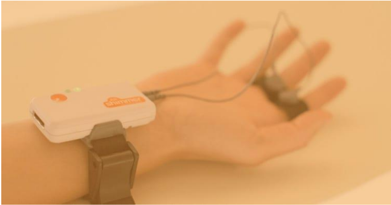
Figure 19 Image shows GSR tool on a study participant. Image source: Bryn Farnsworth (2021): Imotions: What is GSR (galvanic skin response) and how does it work?
