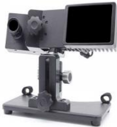
Figure 28 Showing EyeLink 1000 Plus to capture eye tracking data as stimuli is displayed on the screen and set up in actual lab used for the current study
