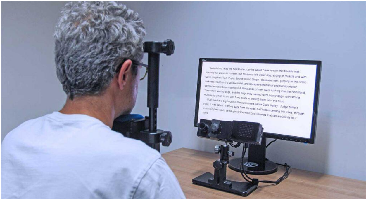
Figure 27 Showing how participants are positioned on to head brace for EyeLink 1000 Plus to capture eye tracking data as stimuli is displayed on the screen.
