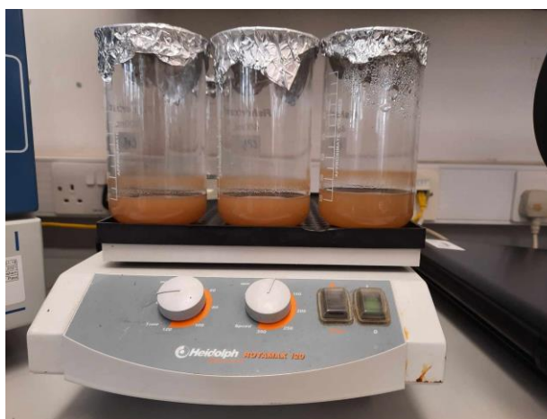
Figure 3.3 - Samples immersed in approximately 20 ml zinc chloride solution, left to be agitated on the orbital shaker for 12 hours.
