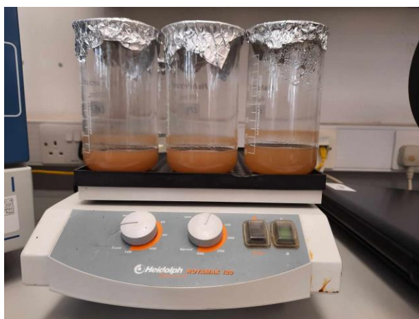
SOP Figure 2.2 - Samples immersed in zinc chloride solution and agitated on orbital shaker
