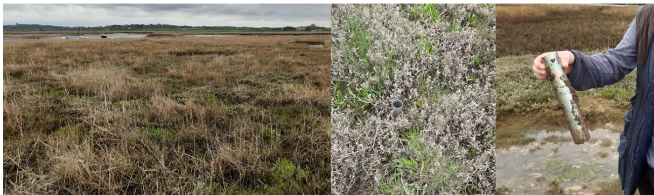
Figure 2.6 - Initial salt marsh samples, showing; salt marsh location (left), core knocked into the ground (mid), and extracted core containing salt marsh sediment (right).
