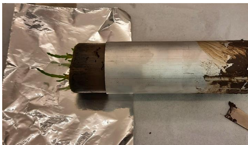
SOP Figure 2.1 - Sediment sample being pushed out of core in preparation for slicing
