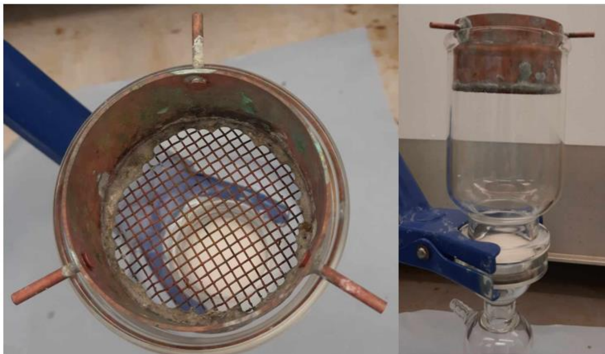
Figure 2.12 - Custom made brass sieve, shown set-up and sitting in filtration apparatus.
