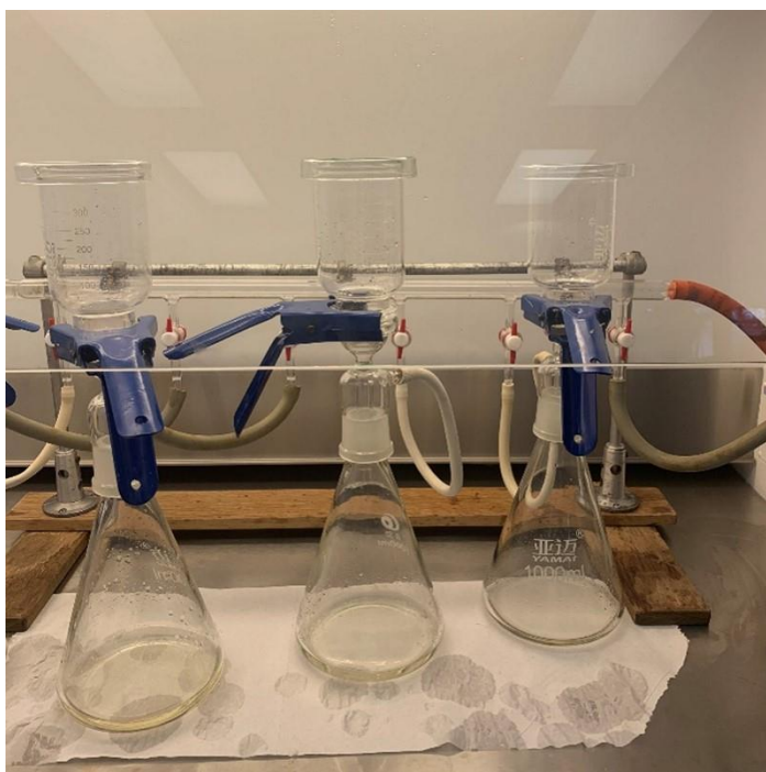
SOP Figure 1.3 - Glass filtering apparatus used to filter all solutions. Buncher flask, filter holder, filter funnel, petri dish to cover funnel and clamp shown.
