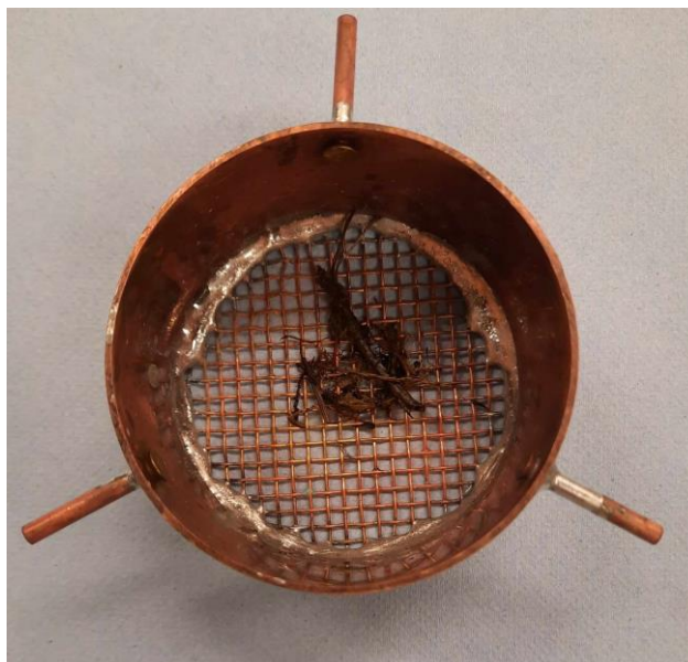
Figure 3.6 - Custom metal sieve piece, shown detached from glassware apparatus, containing larger vegetation pieces that have been sieved off.
