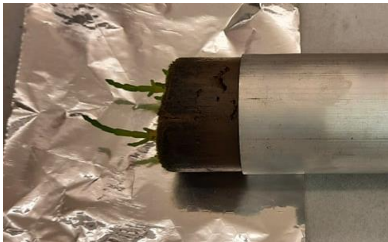
Figure 3.2 - Mud being extracted from the corer, showing top few centimetres of sediment (and surface vegetation) having been pushed up and out of the corer
